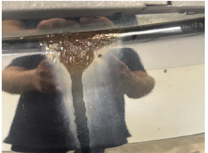
12: Boot Lid Rusted Over 5mm
