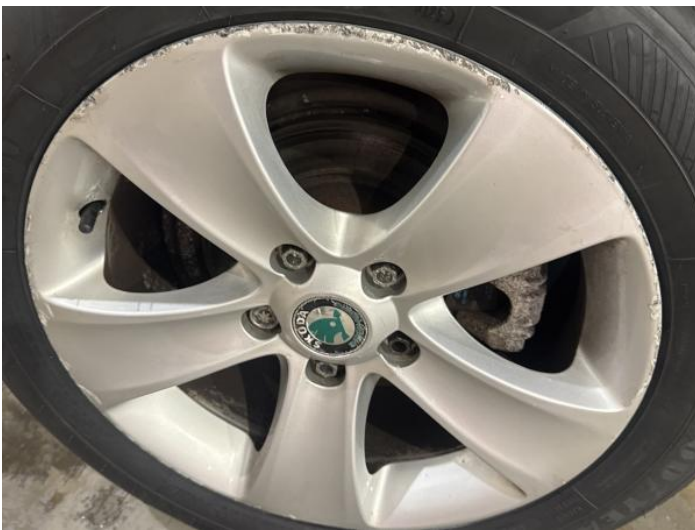
11: Wheel osr Scratched Over 50mm
