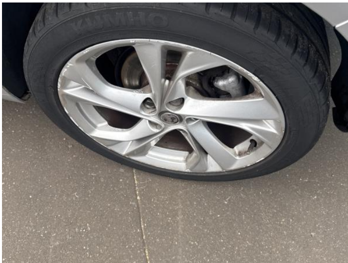
3: Wheel nsr Scratched Over 50mm
