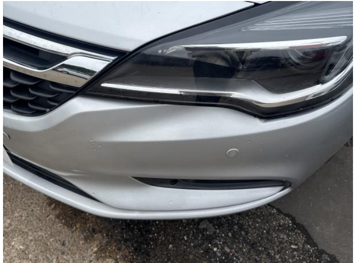
10: Bumper Front Cracked UpTo 25mm
