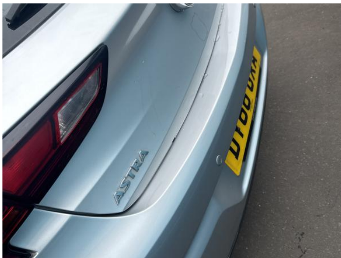
1: Bumper Rear Scratched 25 to 100mm Thru Paint
