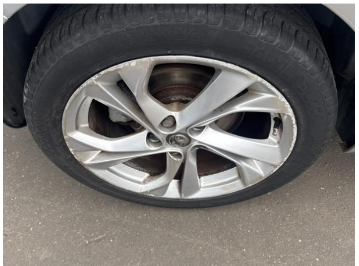
14: Wheel osr Scratched Over 50mm
