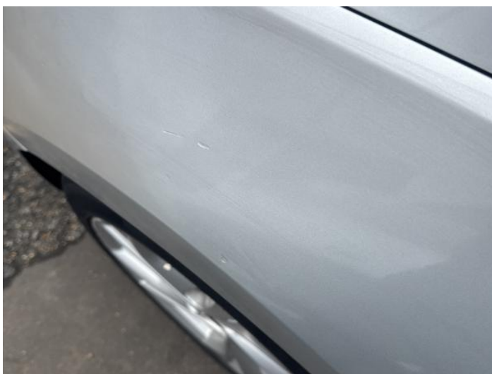
7: Wing nsf Poor Previous Repair Poor Paint
