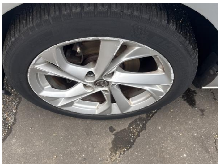
8: Wheel nsf Scratched Over 50mm
