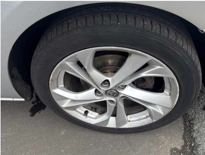
11: Wheel osf Scratched Over 50mm
