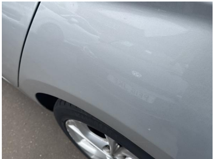
4: Qtr Panel nsr Dented Over 2 UpTo 10mm
