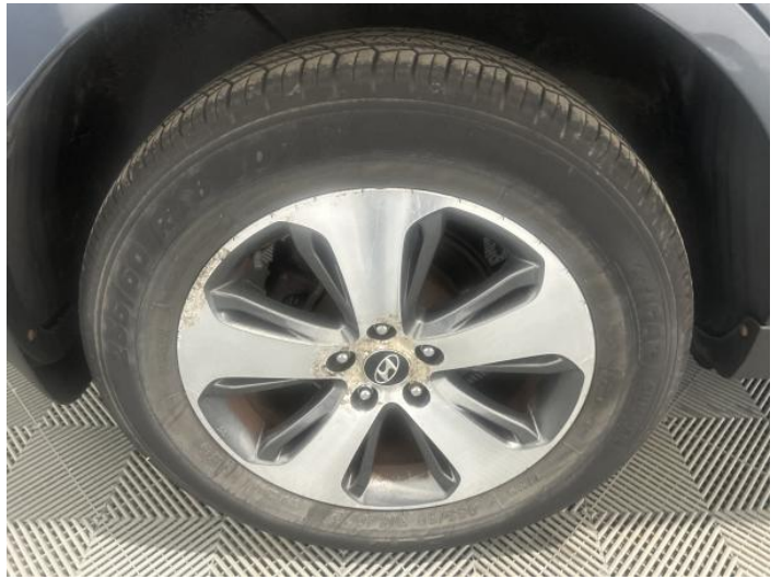
6: Wheel osr Corroded Light
