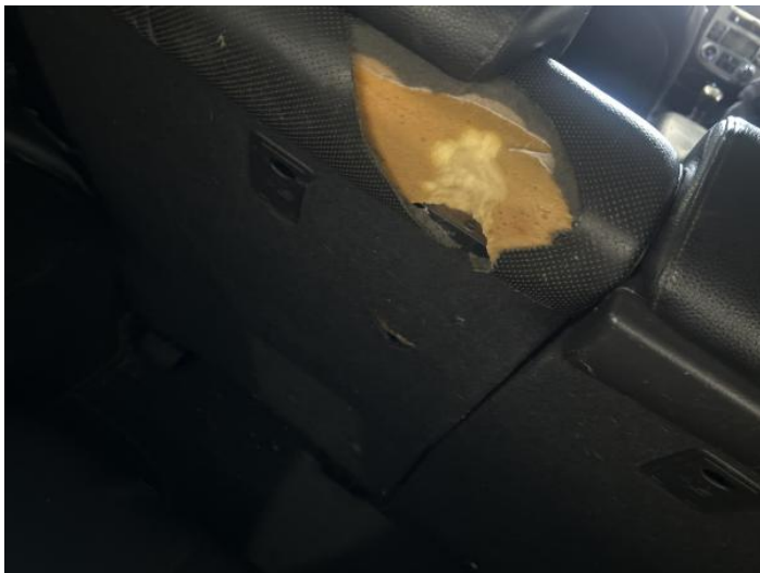
21: Seat Back Cover nsr Holed Over 3mm
