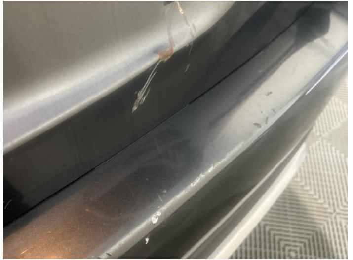
10: Tailgate Dented With Paint Damage
