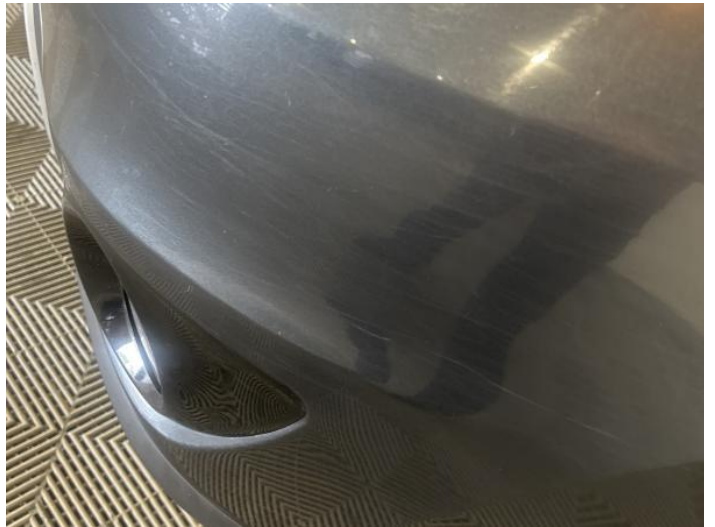
18: Bumper Front Scratched Over 25mm Not Thru Paint
