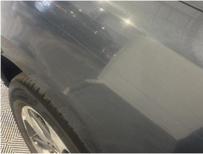
15: Wing nsf Scratched Over 25mm Not Thru Paint
