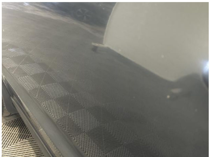
14: Door nsf Scratched Over 25mm Not Thru Paint
