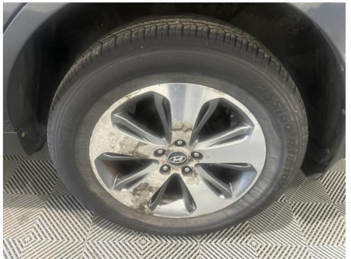
12: Wheel nsr Corroded Light
