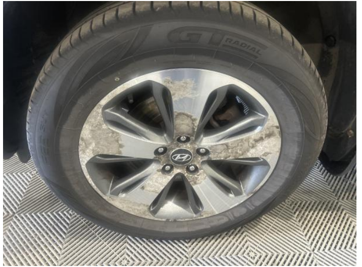
16: Wheel nsf Corroded Light
