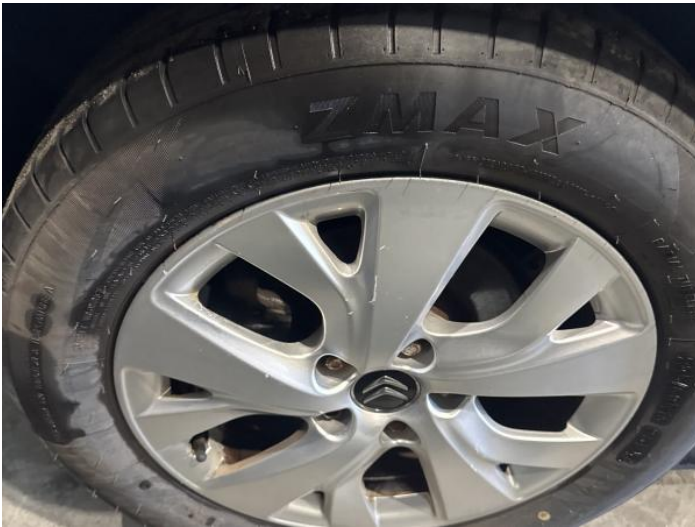
11: Wheel osr Scratched Over 50mm
