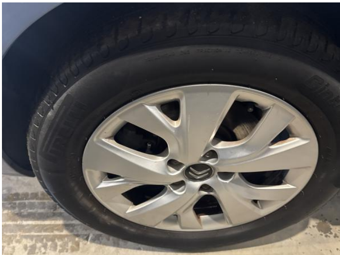
3: Wheel nsf Scratched Up To 50mm
