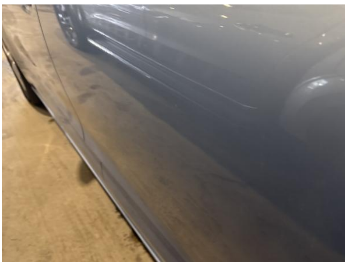
7: Door nsr Dented With Paint Damage
