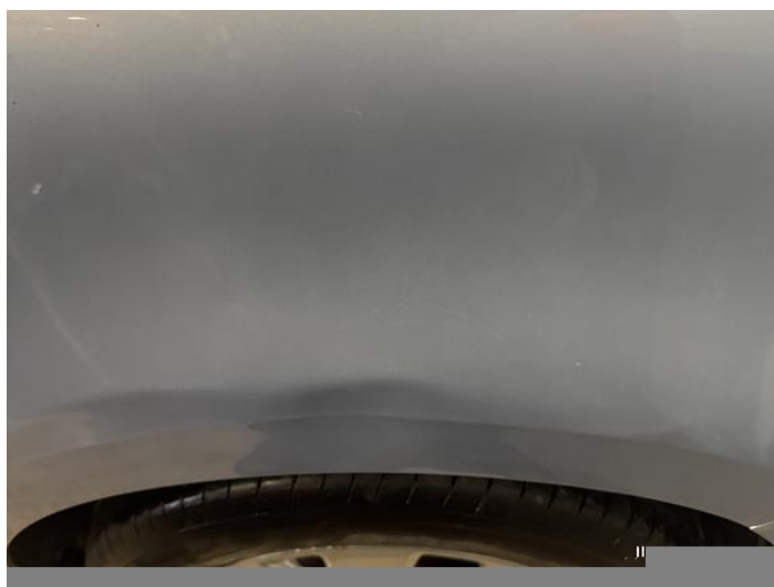
8: Qtr Panel nsr Dented Over 30mm
