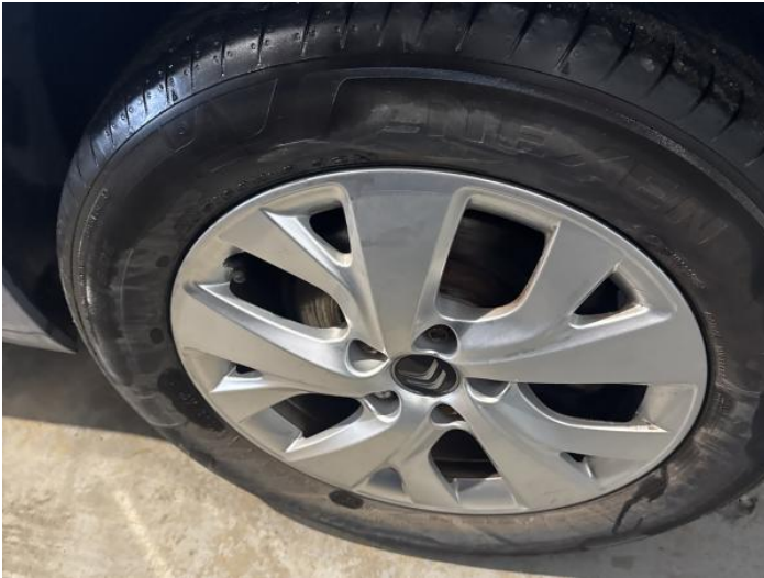
9: Wheel nsr Corroded Light
