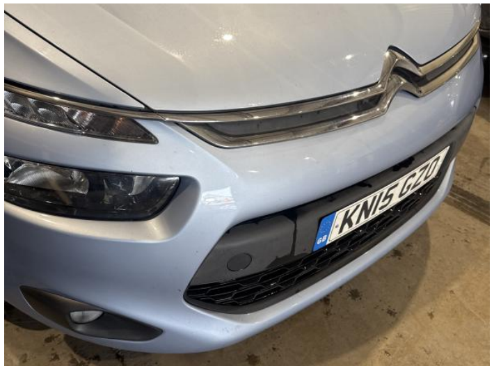
2: Bumper Front Chipped Multiple Chips
