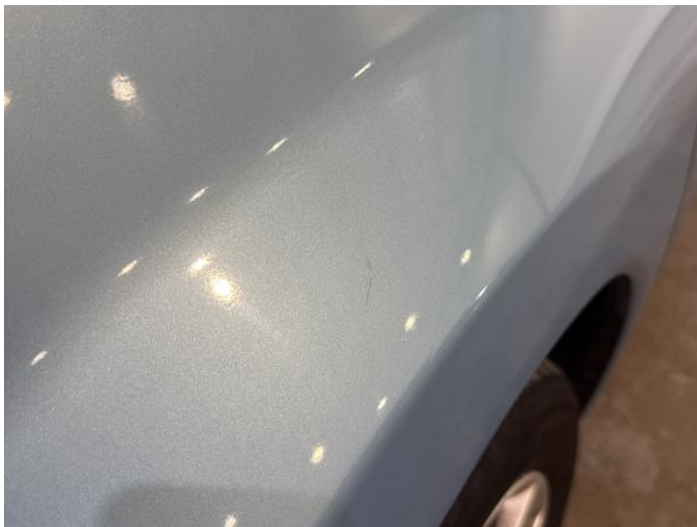
3: Wing nsf Scratched UpTo 25mm Thru Paint
