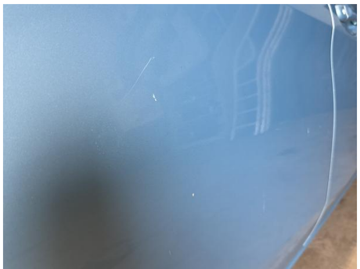
12: Door osr Scratched Over 25mm Thru Paint
