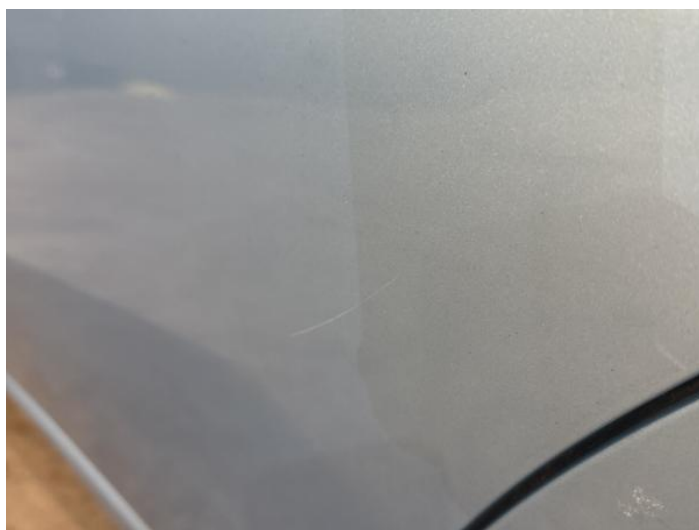
8: Door nsr Scratched Over 25mm Thru Paint
