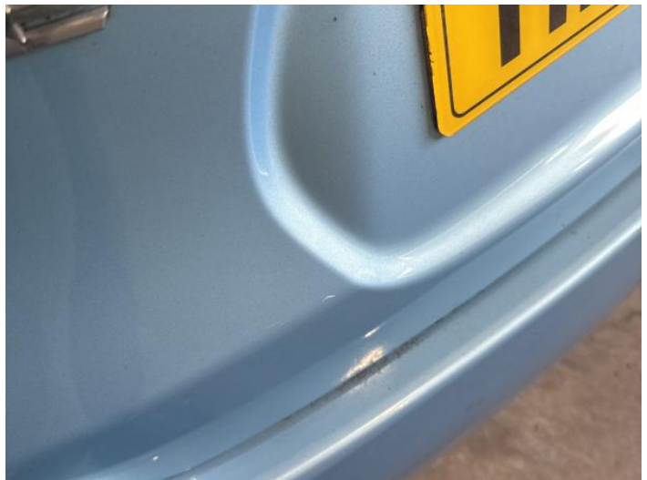
10: Tailgate Scratched UpTo 25mm Thru Paint
