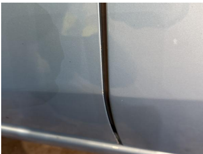
7: Door nsf Chipped Edge Chip
