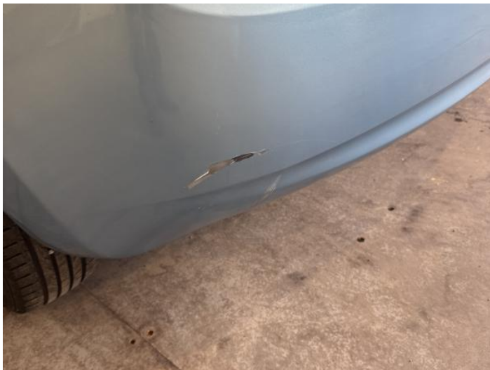
9: Bumper Rear Scratched Over 100mm Thru Paint
