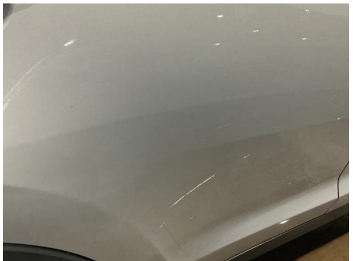
14: Door osr Dented With Paint Damage
