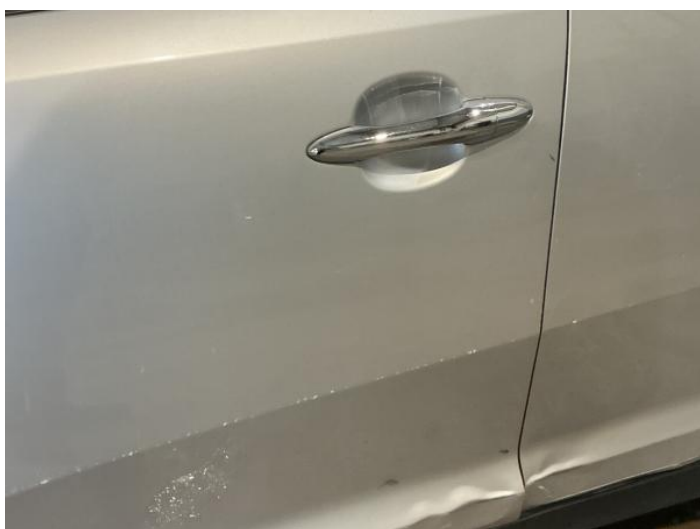
5: Door nsf Dented With Paint Damage
