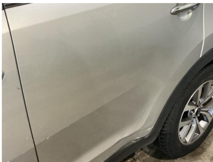
6: Door nsr Dented With Paint Damage
