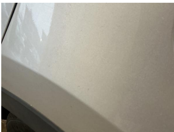
7: Qtr Panel nsr Chipped 1 To 5
