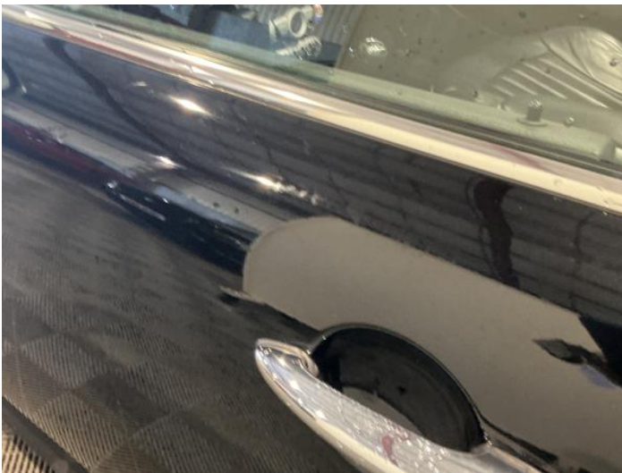
5: Door nsf Poor Previous Repair Poor Paint
