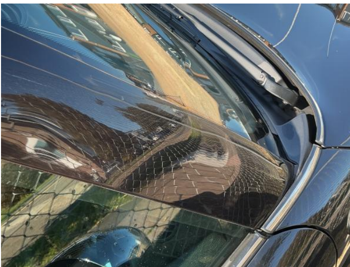
19: A Post os Dented Over 30mm
