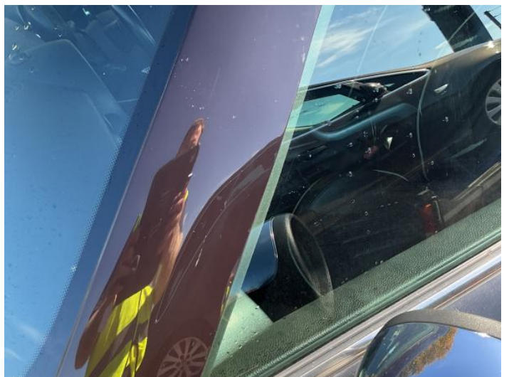
20: A Post ns Dented Over 30mm
