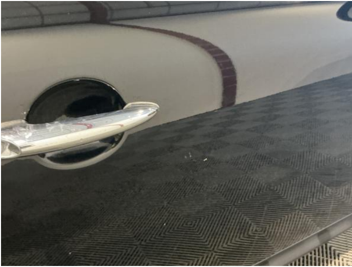
15: Door osf Dented With Paint Damage
