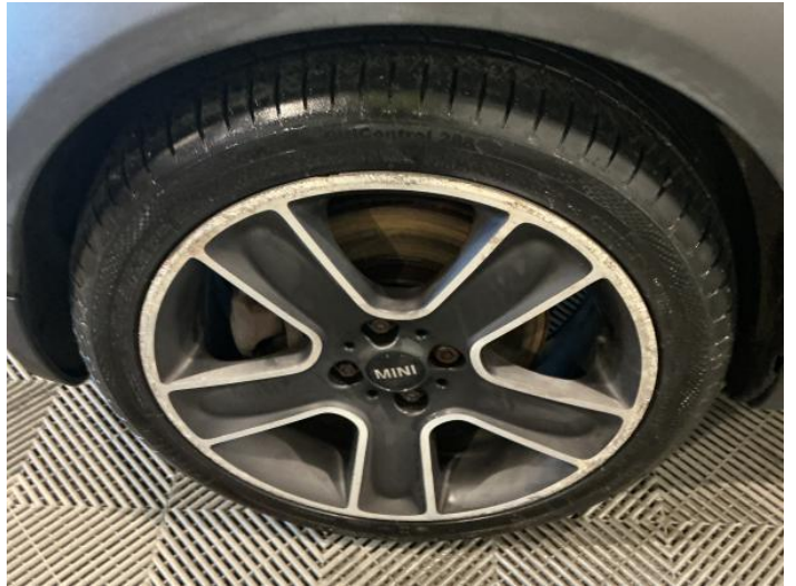
4: Wheel nsf Scratched Over 50mm
