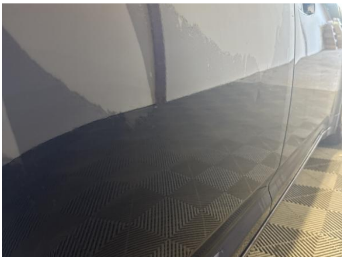
15: Door osr Dented Over 30mm
