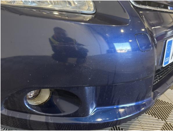
3: Bumper Front Dented With Paint Damage
