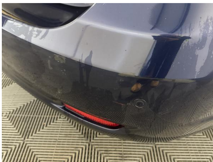
12: Bumper Rear Scratched Over 100mm Thru Paint
