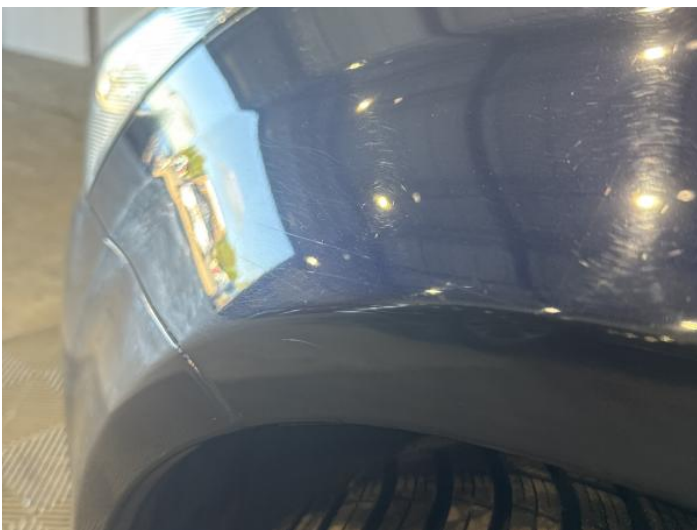
7: Wing nsf Scratched UpTo 25mm Thru Paint
