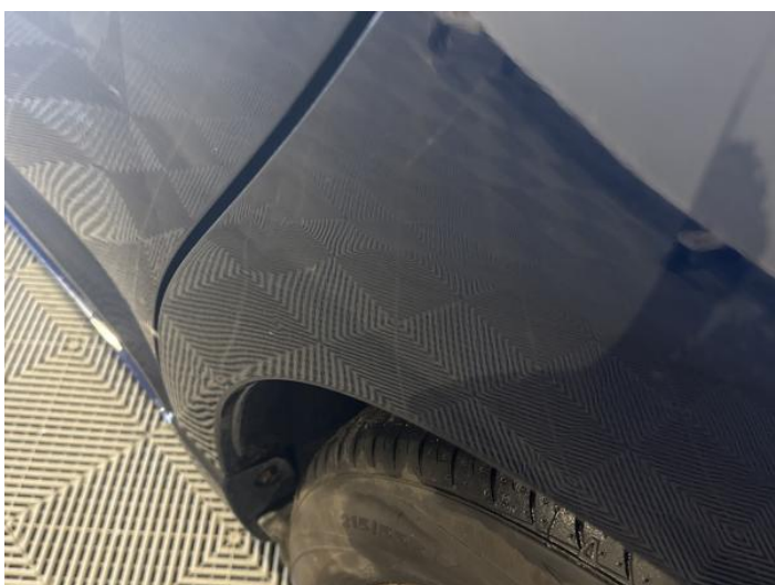
11: Qtr Panel nsr Dented Between 10mm + 30mm
