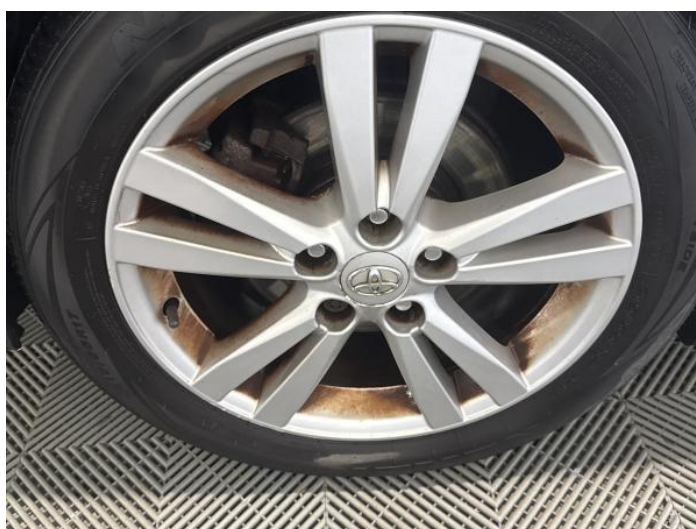
14: Wheel osr Scratched Up To 50mm
