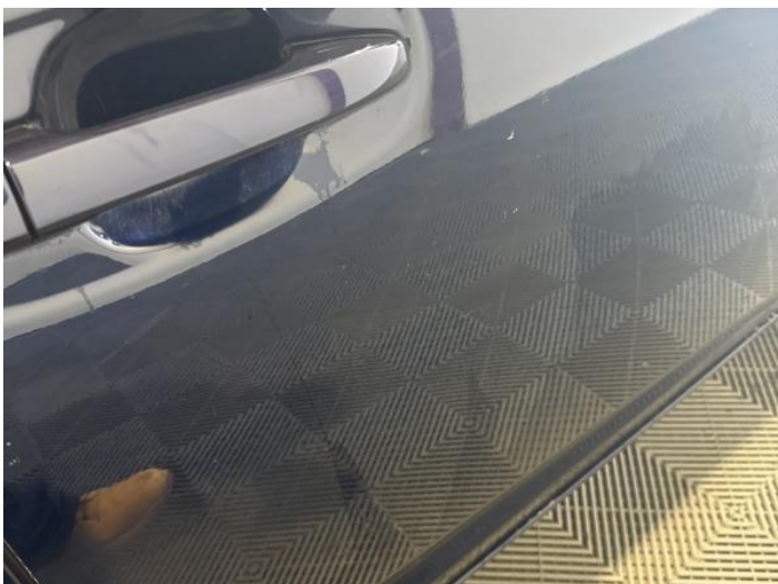
16: Door nsf Scratched Over 25mm Thru Paint
