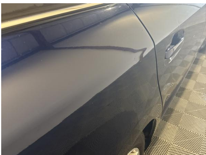
13: Qtr Panel osr Dented Over 30mm
