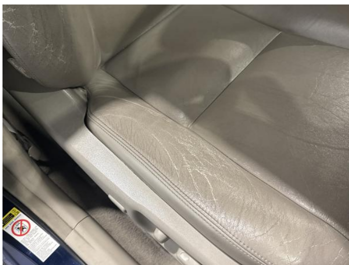
1: Seat Base Cover osf Scuffed Over 25mm
