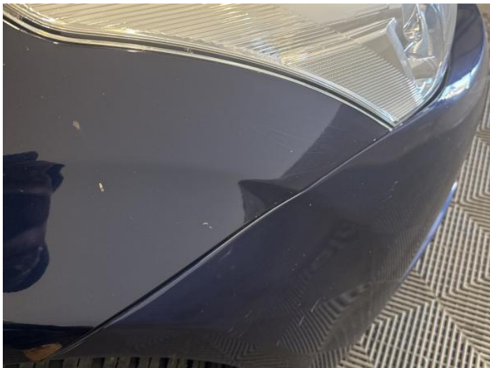
17: Wing osf Scratched Over 25mm Thru Paint
