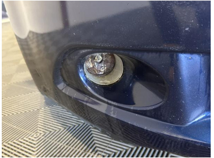
4: Fogdriving Lamp osf Broken Replace
