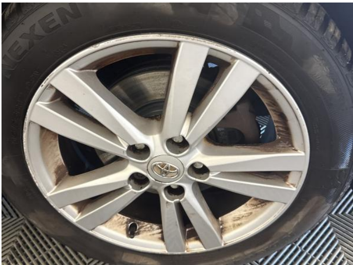
18: Wheel osf Scratched Over 50mm
