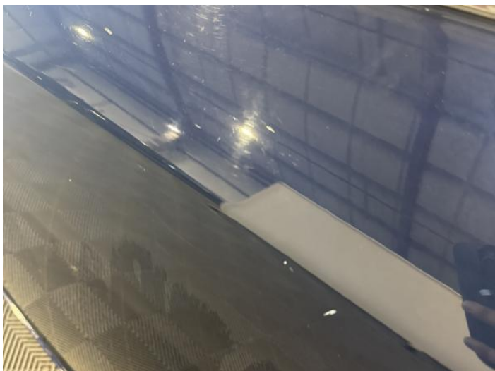
9: Door nsr Scratched Over 25mm Thru Paint
