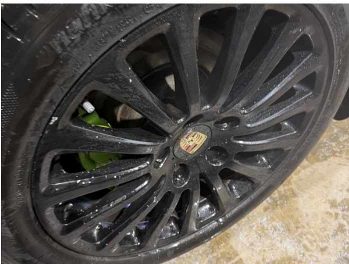
13: Wheel osr Scratched Up To 50mm
