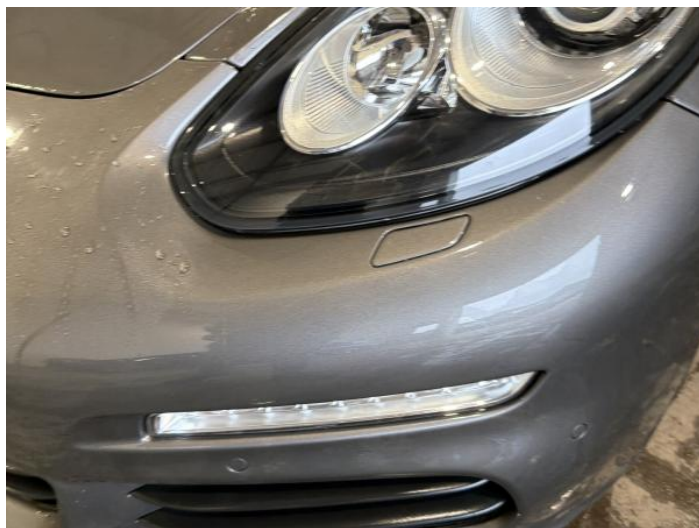
2: Bumper Front Chipped Multiple Chips
