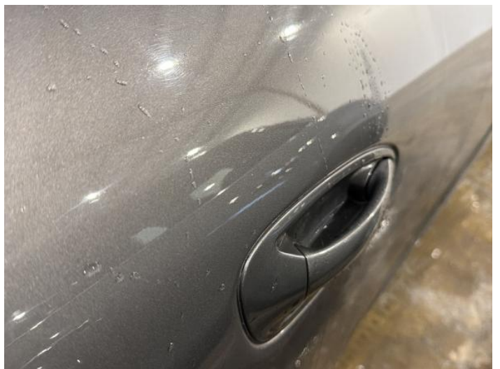
14: Door osr Poor Previous Repair Poor Paint
