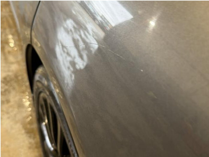
9: Qtr Panel nsr Dented Over 2 UpTo 10mm
