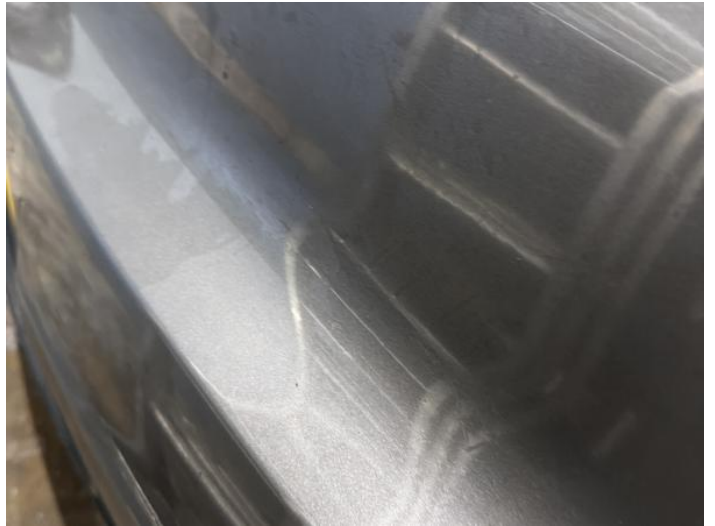
10: Bumper Rear Chipped Multiple Chips
