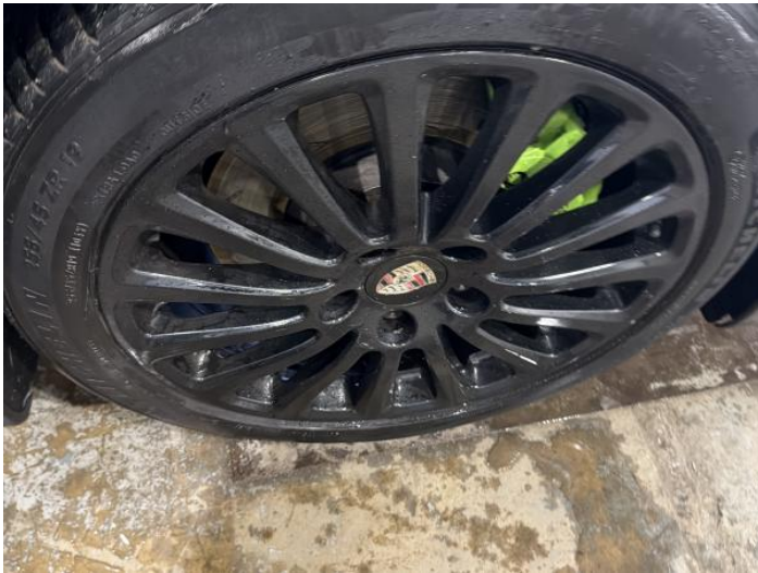
18: Wheel osf Scratched Up To 50mm
