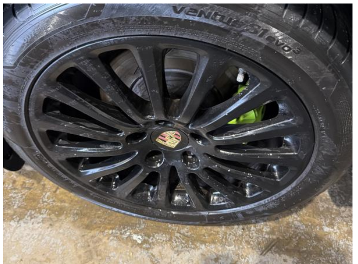
8: Wheel nsr Scratched Up To 50mm
