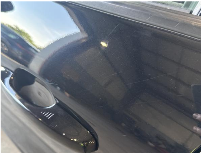
5: Door nsf Scratched UpTo 25mm Thru Paint
