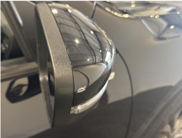
11: Door Mirror Assy osf Scratched (Painted) UpTo 25mm Thru Paint
