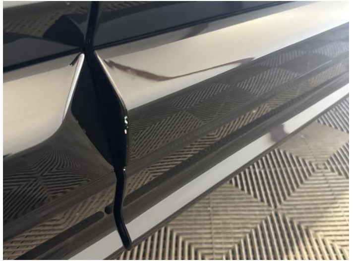
10: Door Moulding osf Scratched (Painted) UpTo 25mm Thru Paint
