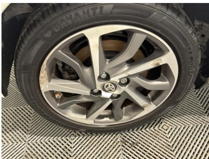
11: Wheel osr Scratched Over 50mm
