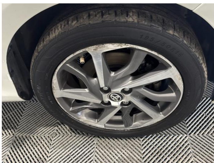
14: Wheel osf Scratched Over 50mm
