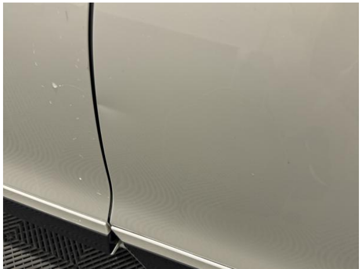
6: Door nsr Dented Over 30mm
