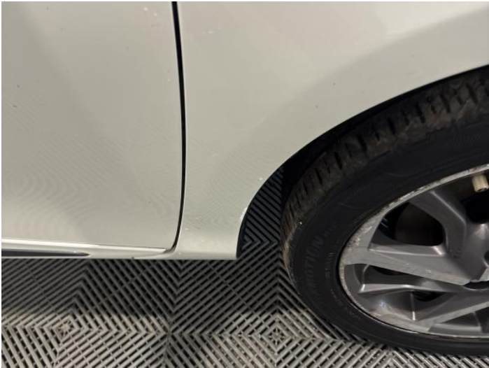
15: Wing osf Dented With Paint Damage
