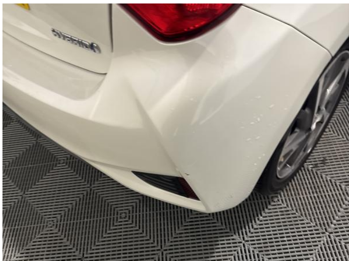
9: Bumper Rear Scratched Over 100mm Thru Paint
