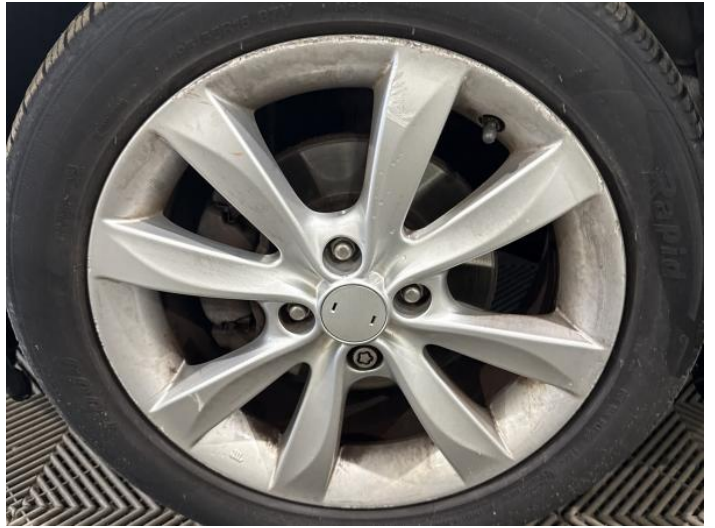
4: Wheel nsf Scratched Over 50mm
