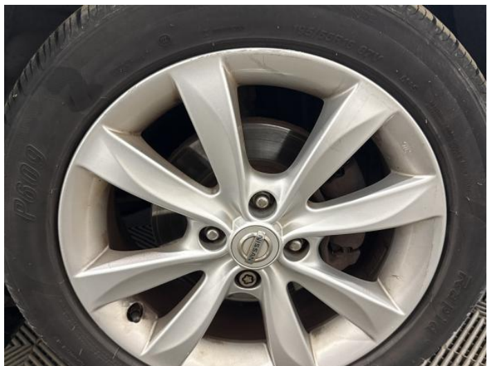
14: Wheel osf Scratched Over 50mm
