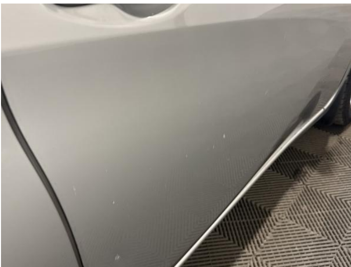
13: Door nsf Dented Over 30mm
