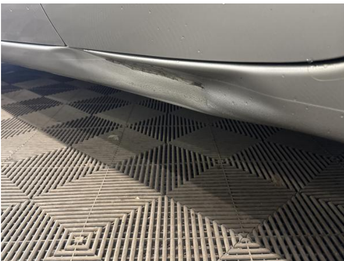
7: Sill ns Dented With Paint Damage
