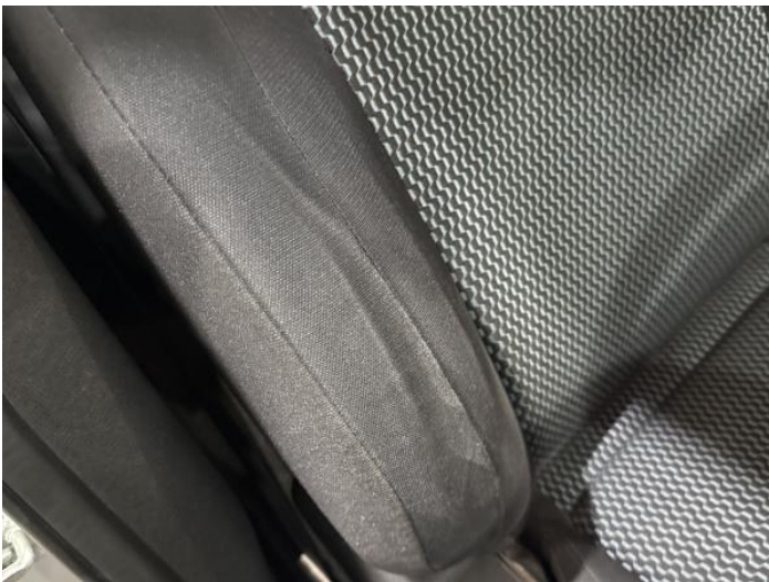
1: Seat Back Cover osf Scuffed Over 25mm
