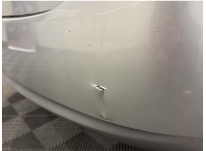
10: Bumper Rear Cracked UpTo 25mm
