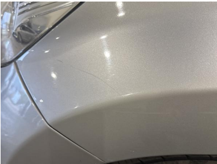
5: Wing nsf Scratched Over 25mm Thru Paint
