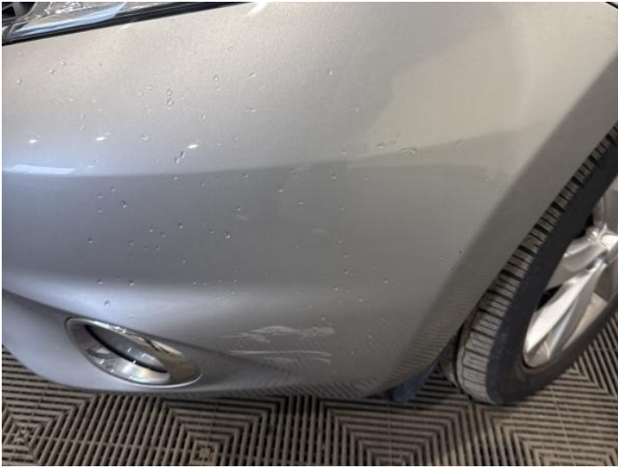
3: Bumper Front Scratched 25 to 100mm Thru Paint
