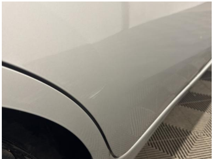
12: Door osr Scratched Over 25mm Thru Paint
