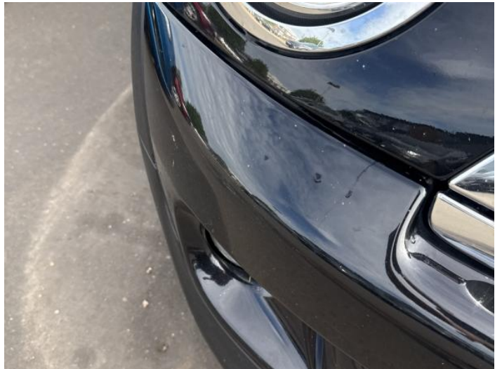
2: Bumper Front Scratched 25 to 100mm Thru Paint
