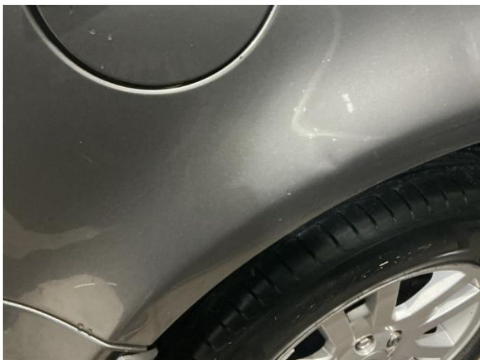
3: Qtr Panel osr Dented With Paint Damage
