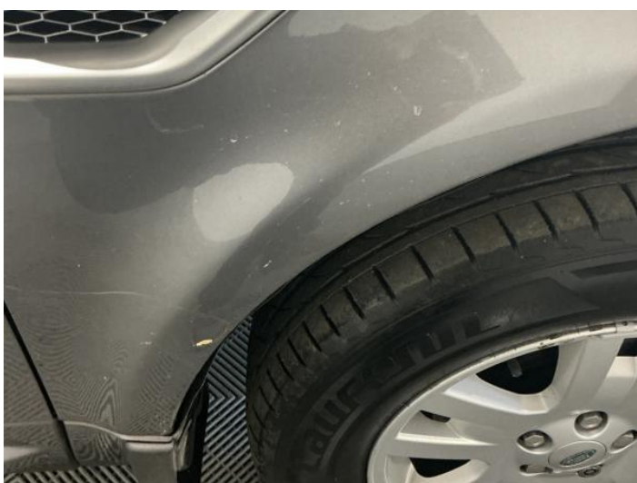
7: Wing osf Scratched Over 25mm Thru Paint
