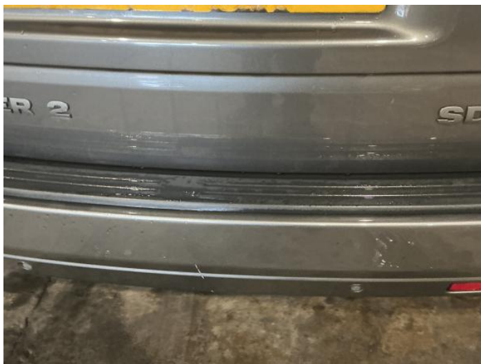
1: Bumper Rear Scratched Over 100mm Thru Paint
