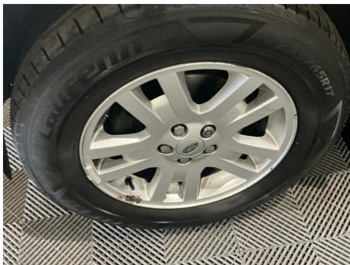
12: Wheel nsf Corroded Light
