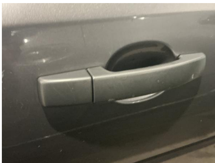
6: Door osf Chipped Multiple Chips
