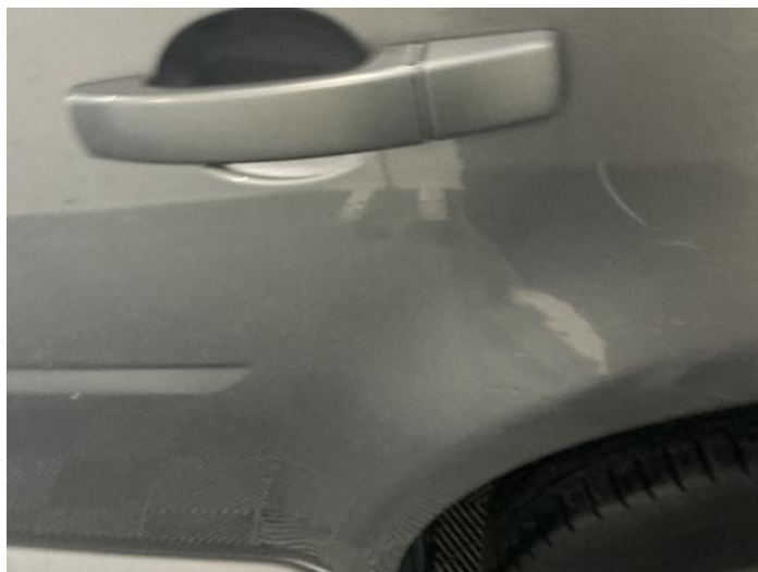
16: Door nsr Scratched Over 25mm Not Thru Paint
