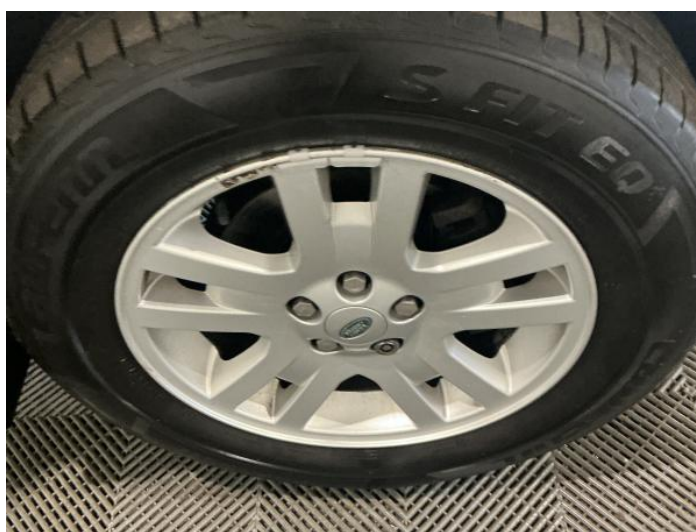
8: Wheel osf Scratched Over 50mm
