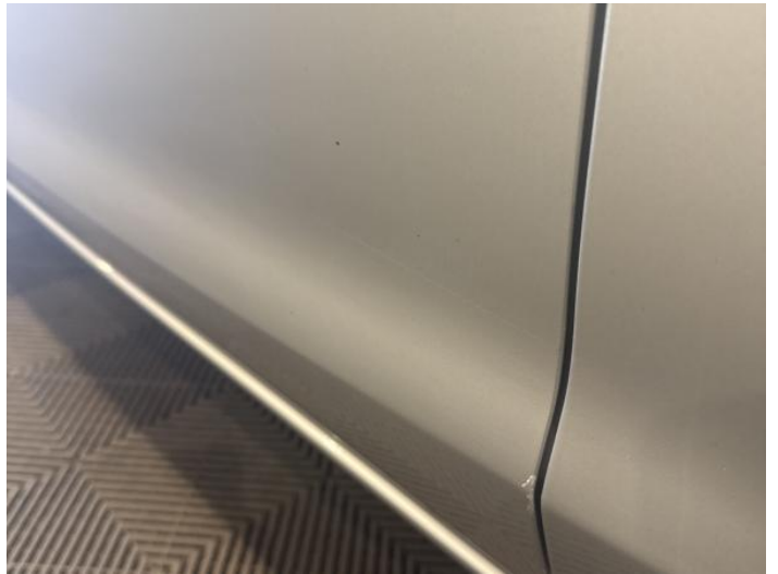
6: Door nsf Scratched Over 25mm Thru Paint
