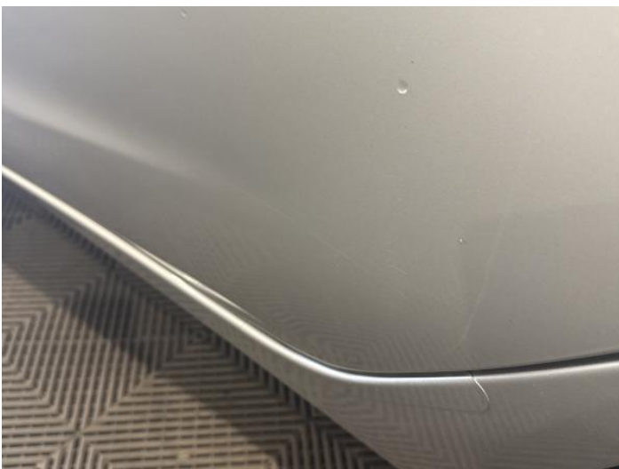
7: Door nsr Scratched Over 25mm Thru Paint
