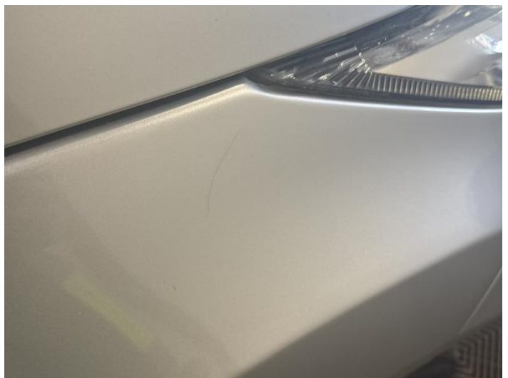
14: Wing osf Scratched Over 25mm Thru Paint
