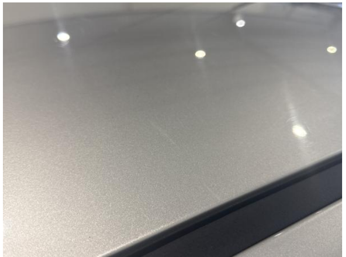
12: Roof Scratched UpTo 25mm Thru Paint
