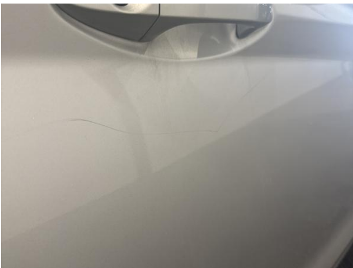
13: Door osf Scratched Over 25mm Thru Paint
