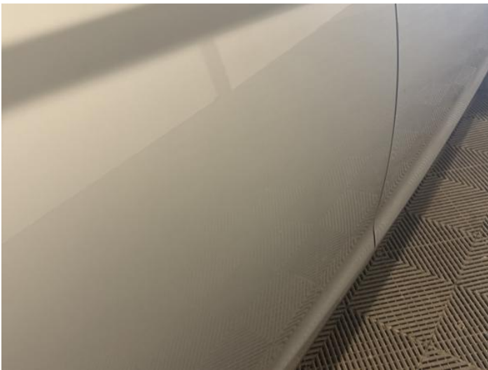
11: Door osr Dented Over 30mm
