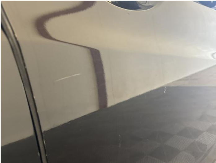
15: Door osf Scratched Over 25mm Thru Paint
