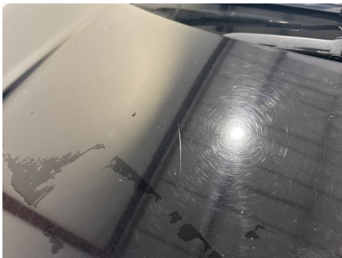
1: Bonnet Scratched Over 25mm Thru Paint
