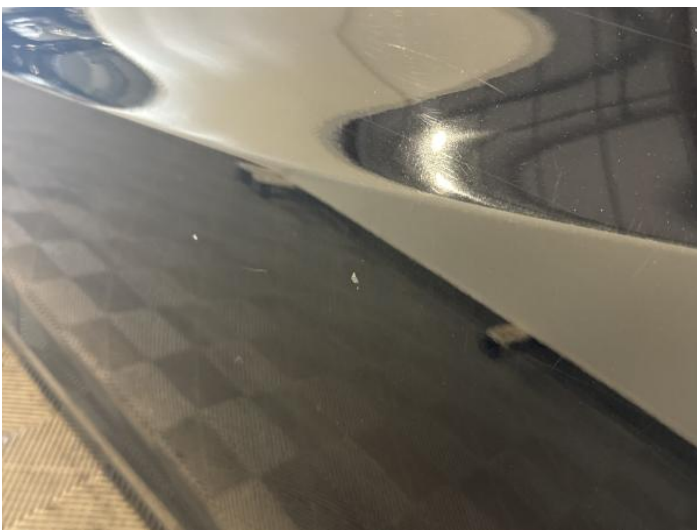
7: Door nsr Dented Between 10mm + 30mm
