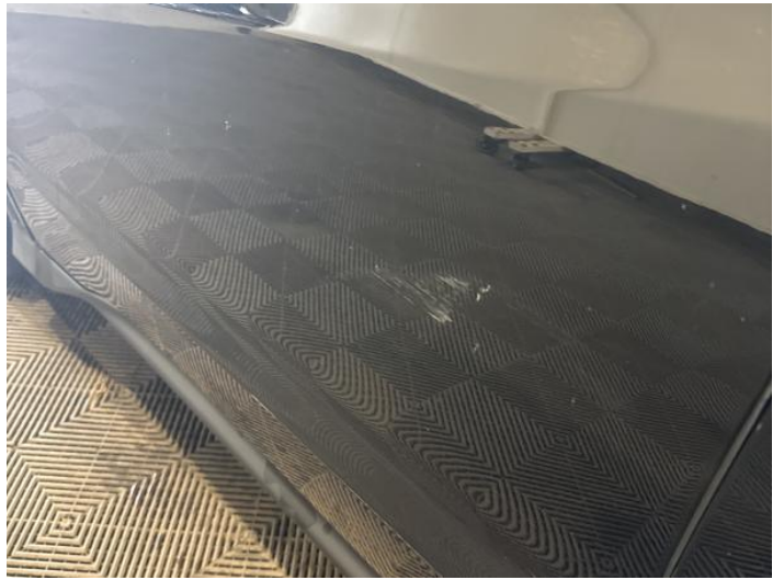
6: Door nsf Scratched Over 25mm Thru Paint
