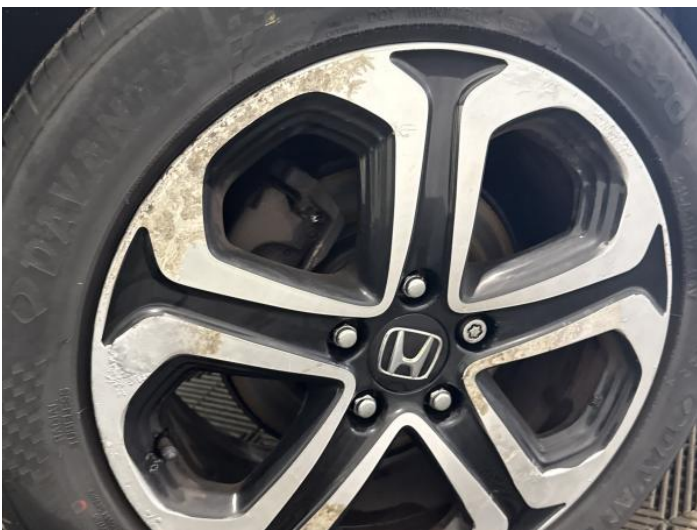
13: Wheel osr Scratched Over 50mm
