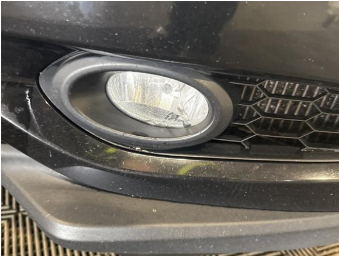
3: Fogdriving Lamp osf Broken Replace
