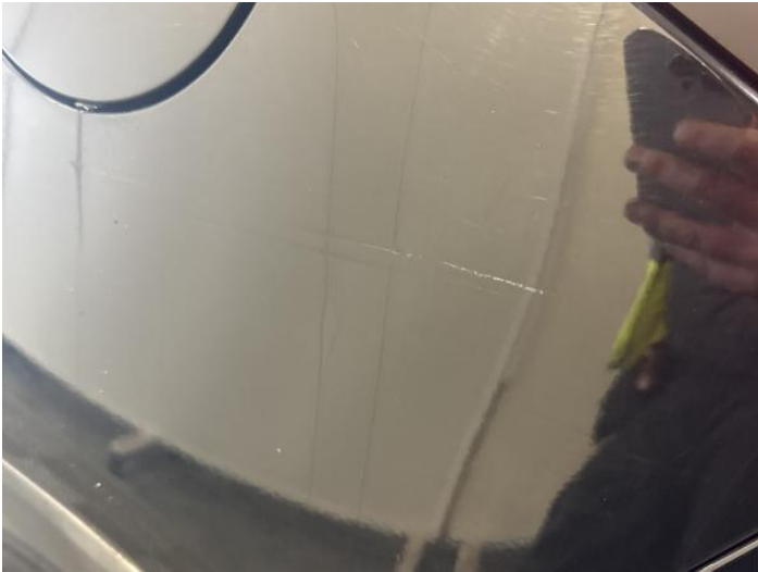
9: Qtr Panel nsr Scratched Over 25mm Thru Paint
