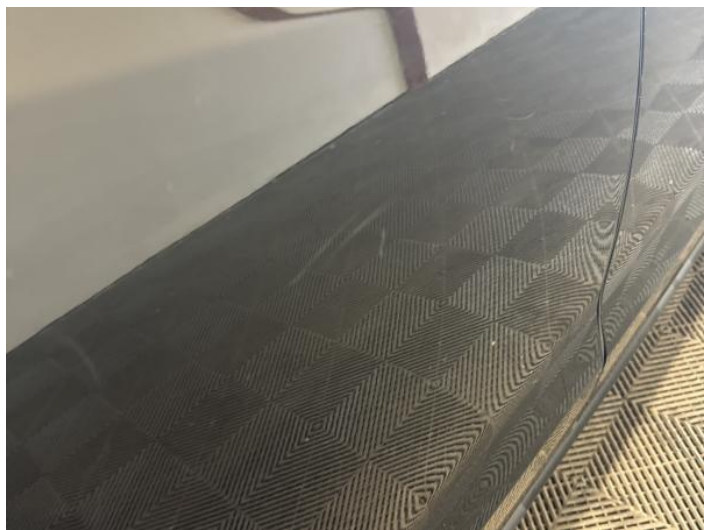
14: Door osr Scratched Over 25mm Thru Paint
