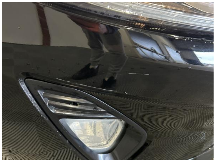
14: Bumper Front Scratched 25 to 100mm Thru Paint
