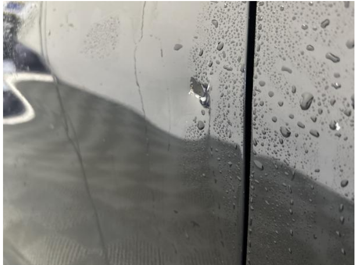
4: Door osf Dented With Paint Damage
