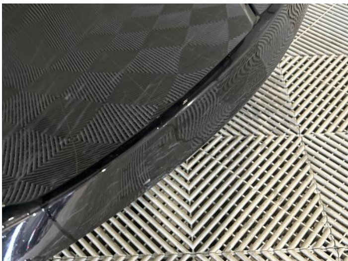
15: Bumper Front Scratched Over 25mm Not Thru Paint
