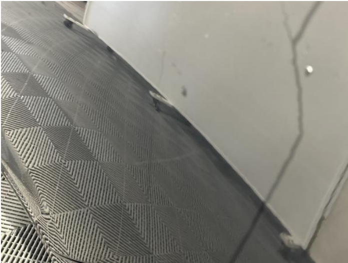
9: Door nsr Scratched Over 25mm Not Thru Paint
