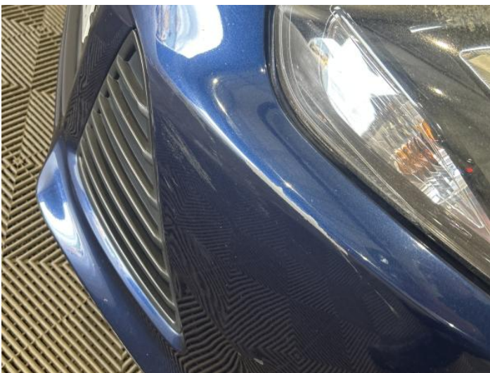
13: Bumper Front Scratched Over 100mm Thru Paint
