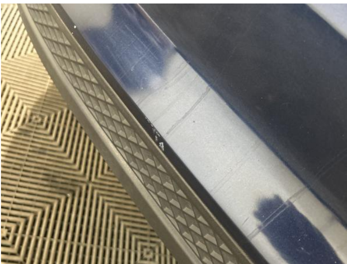
7: Bumper Rear Chipped Multiple Chips
