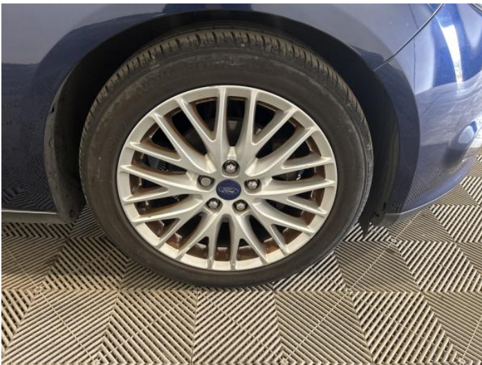
1: Wheel osf Scratched Over 50mm
