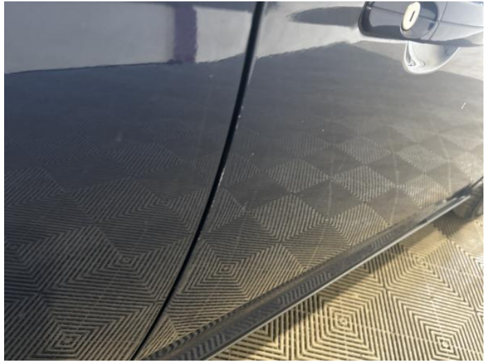
4: Door osf Chipped Edge Chip
