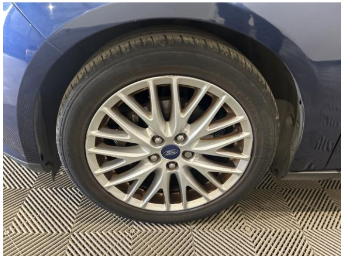
12: Wheel nsf Scratched Up To 50mm
