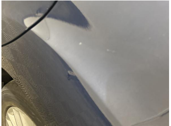
10: Qtr Panel nsr Chipped 1 To 5
