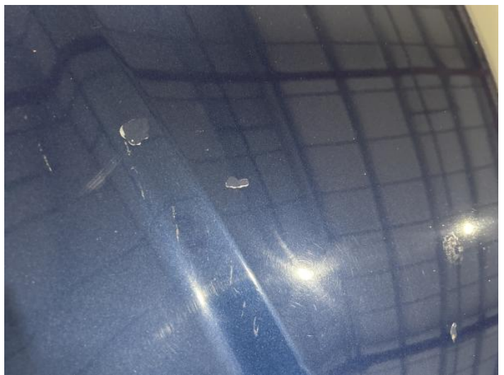
14: Bonnet Poor Previous Repair Paint Flake
