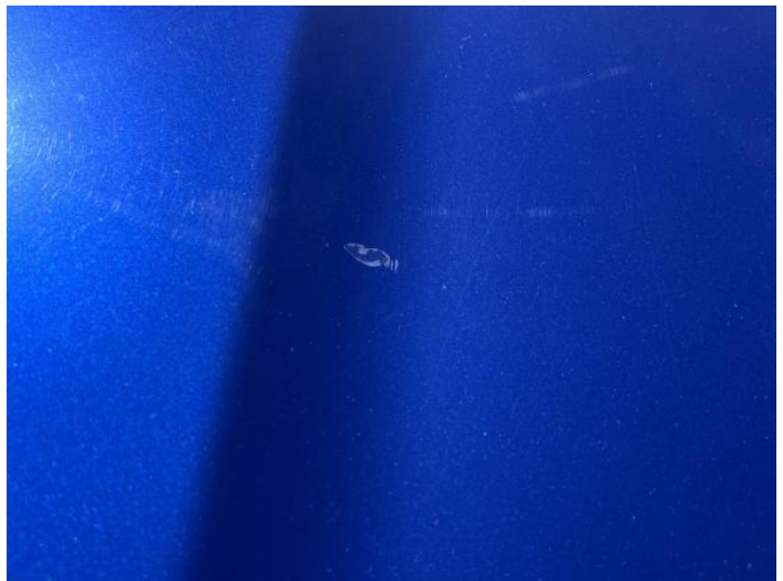
18: Bonnet Poor Previous Repair Paint Flake
