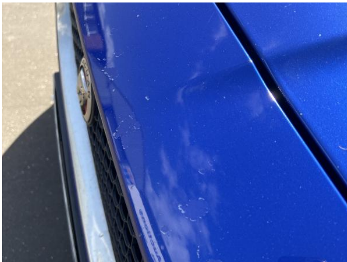
17: Bumper Front Poor Previous Repair Paint Flake
