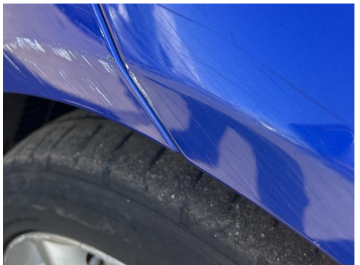
14: Wing nsf Scratched UpTo 25mm Thru Paint
