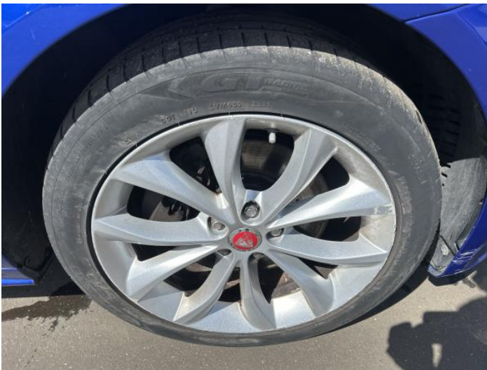
1: Wheel osf Scratched Over 50mm
