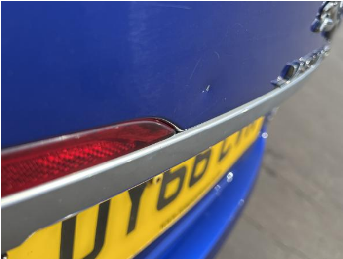
9: Tailgate Dented 2 Or Less UpTo 10mm
