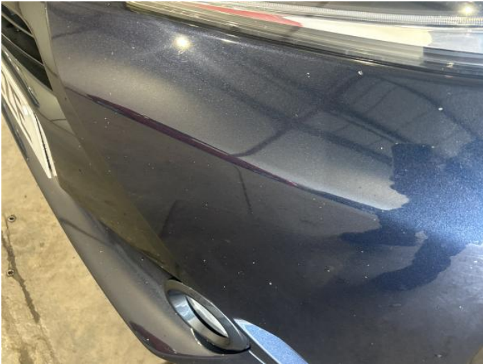
9: Bumper Front Chipped Multiple Chips
