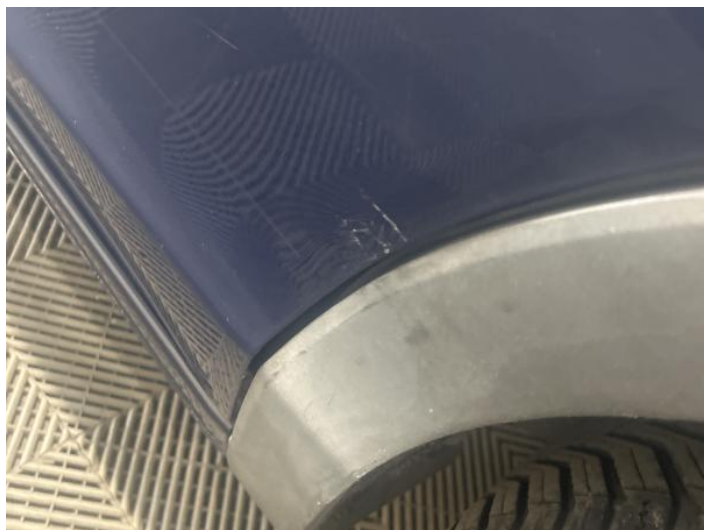
14: Door nsr Scratched UpTo 25mm Thru Paint
