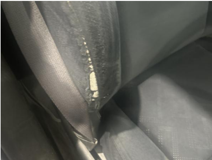
1: Seat Back Cover of Torn Over 3mm
