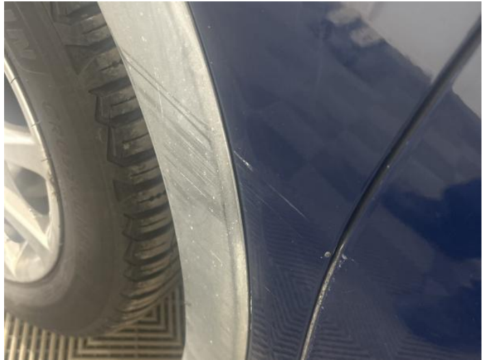
16: Wing nsf Scratched UpTo 25mm Thru Paint
