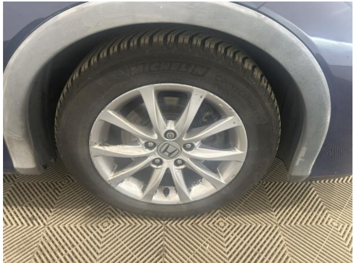
2: Wheel of Corroded Light
