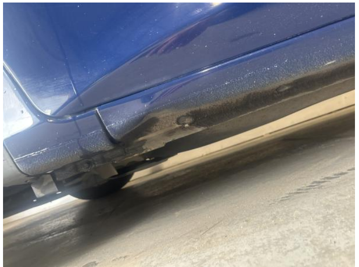
24: Sill ns Dented Over 30mm
