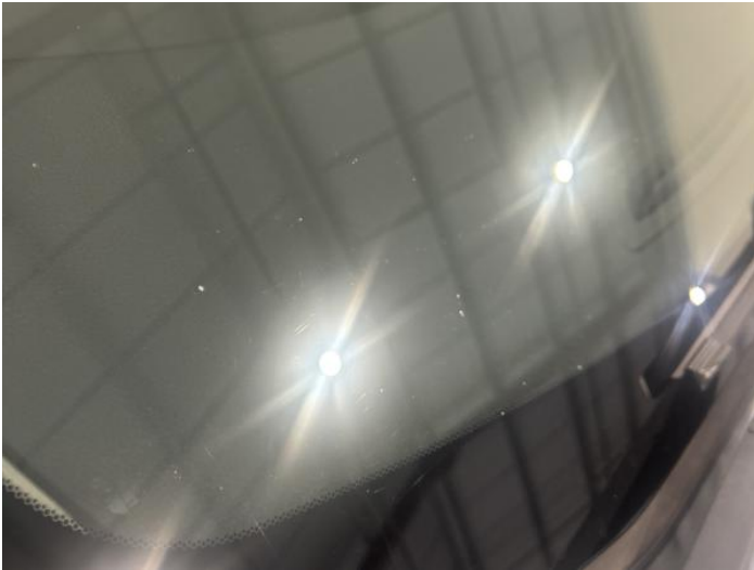
21: Screen Front Chipped UpTo 10mm
