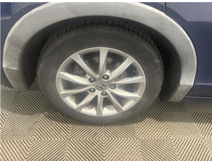
7: Wheel osr Corroded Light
