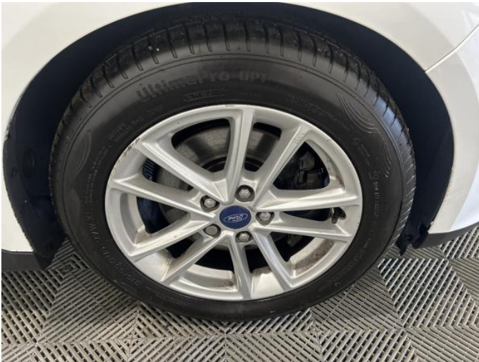
1: Wheel osf Scratched Over 50mm
