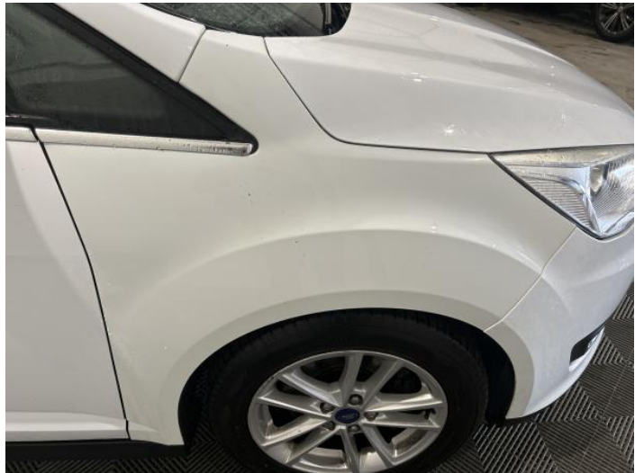
2: Wing osf Poor Previous Repair Poor Colour
