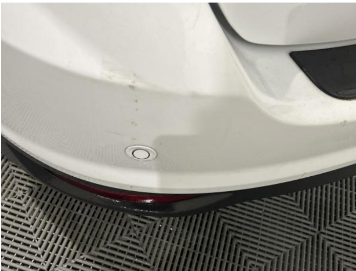
5: Bumper Rear Scratched 25 to 100mm Thru Paint
