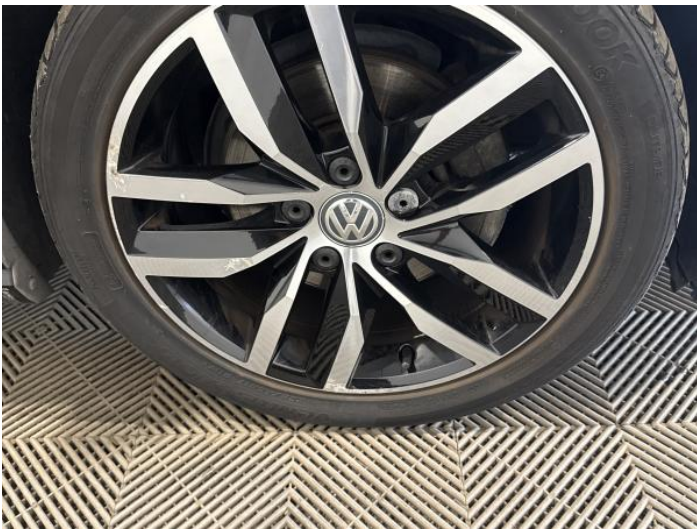
17: Wheel osf Corroded Light
