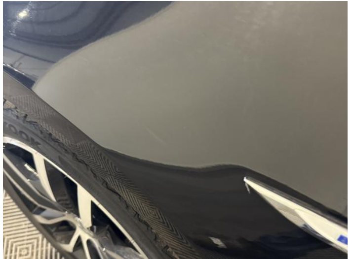
4: Wing nsf Scratched UpTo 25mm Thru Paint
