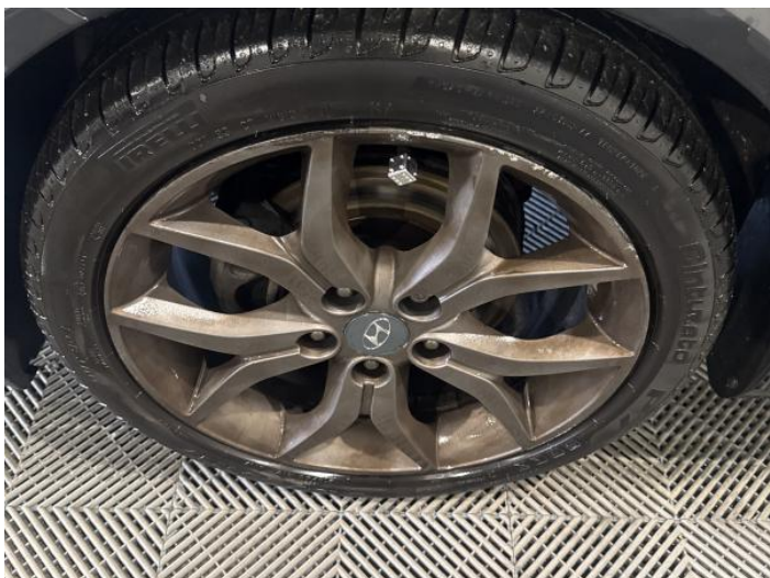
3: Wheel nsf Scratched Over 50mm
