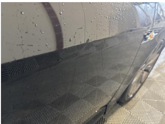
13: Door osf Dented Over 2 UpTo 10mm
