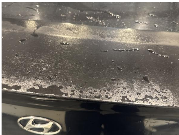
10: Boot Lid Poor Previous Repair Poor Paint
