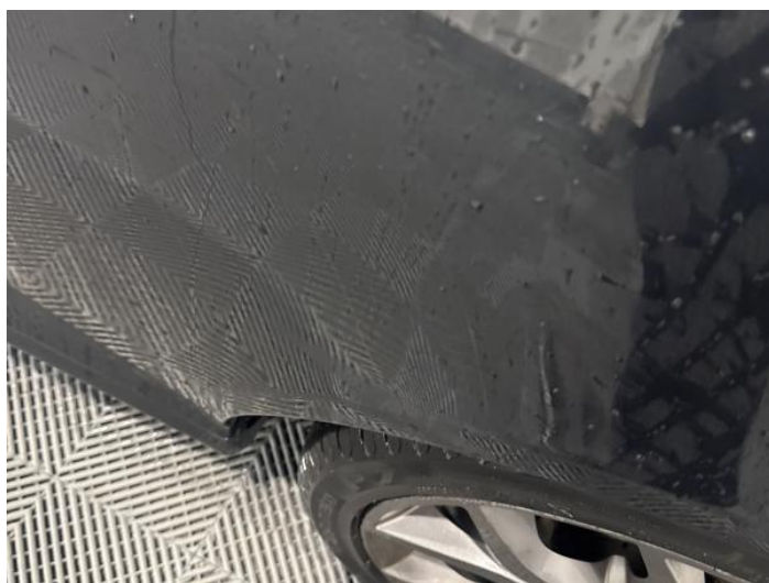
8: Qtr Panel nsr Dented With Paint Damage
