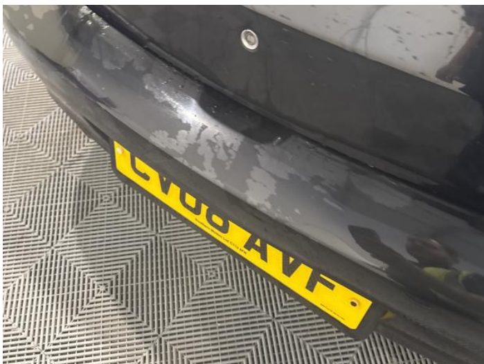
9: Bumper Rear Scratched 25 to 100mm Thru Paint
