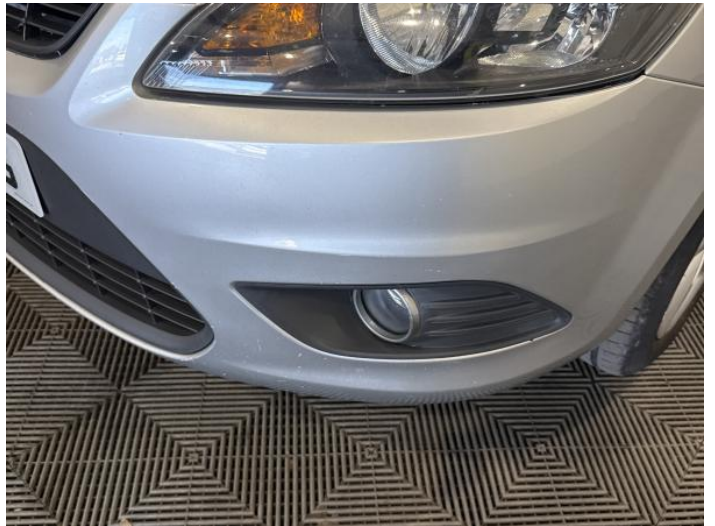
2: Bumper Front Scratched 25 to 100mm Thru Paint
