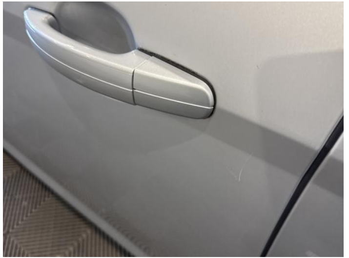
6: Door nsf Scratched Over 25mm Thru Paint
