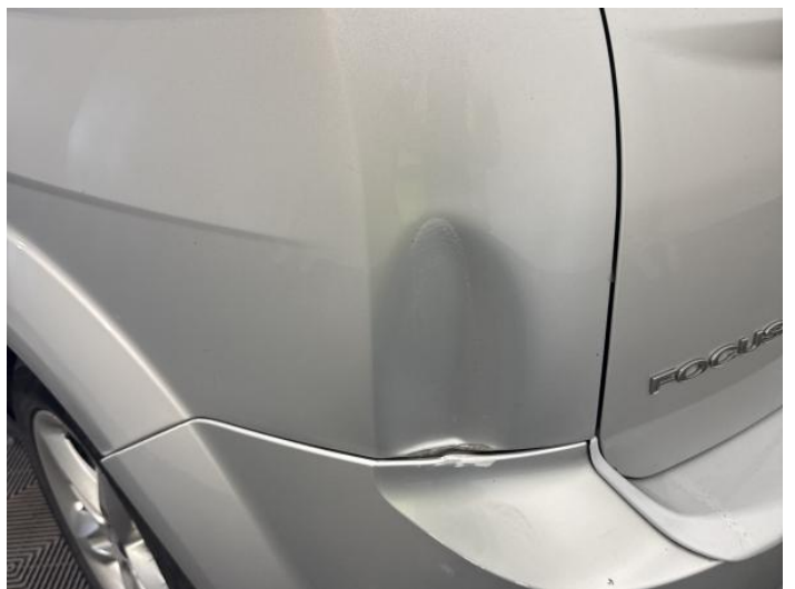
8: Qtr Panel nsr Dented With Paint Damage
