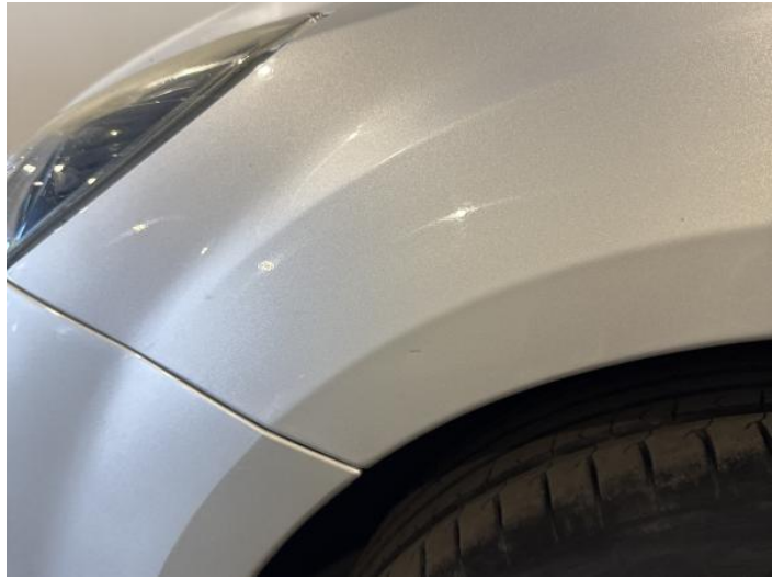
4: Wing nsf Chipped 1 To 5
