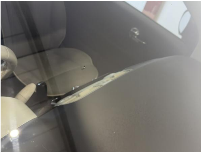
17: Screen Front Chipped UpTo 10mm
