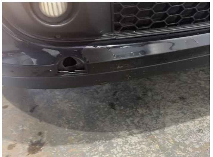
14: Front TowEye Cvr Missing Replace
