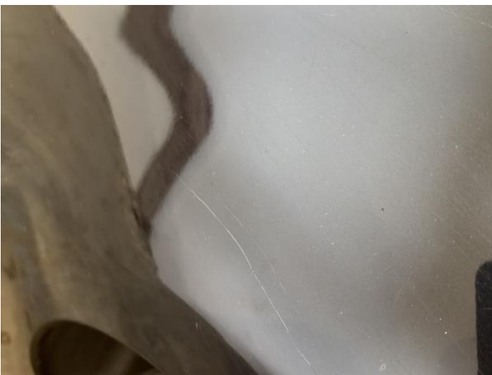
7: Qtr Panel nsr Scratched Over 25mm Thru Paint
