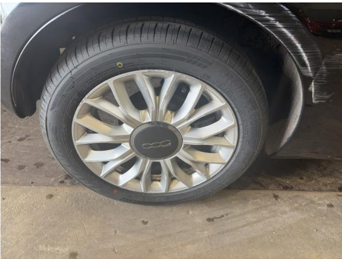
5: Wheel osr Scratched Over 50mm
