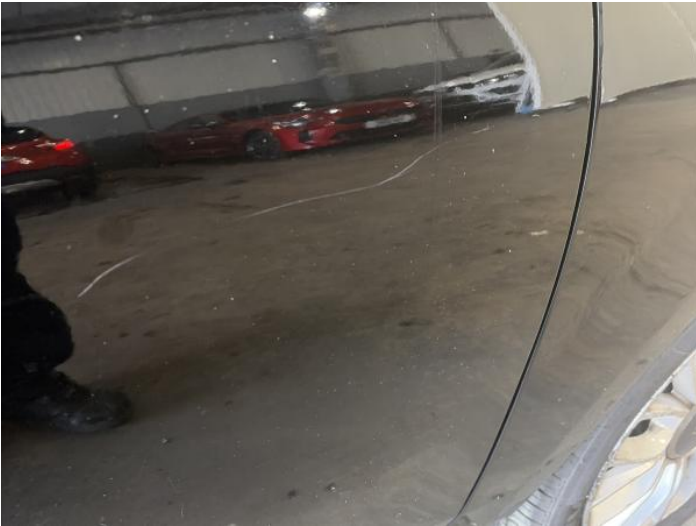
3: Door osf Scratched Over 25mm Thru Paint
