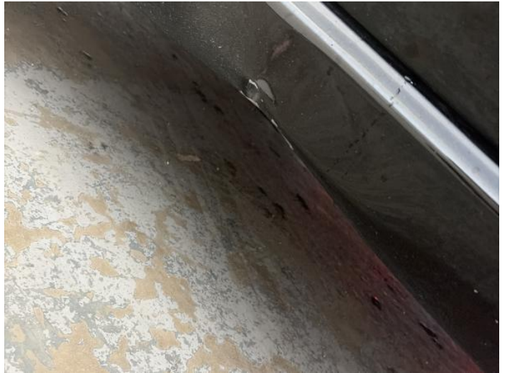
10: Sill ns Dented With Paint Damage
