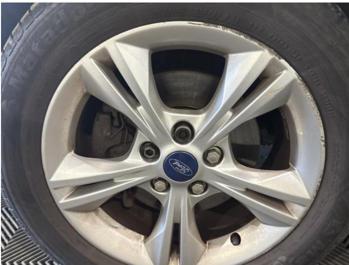
5: Wheel nsf Scratched Over 50mm
