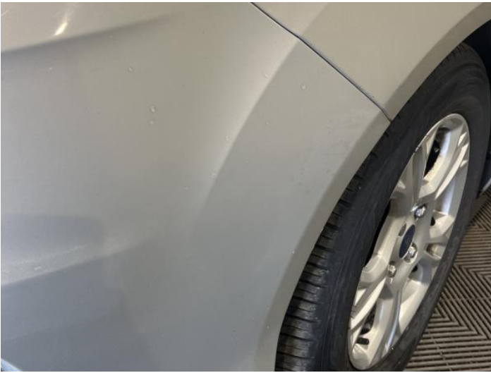
5: Bumper Front Poor Previous Repair Poor Paint
