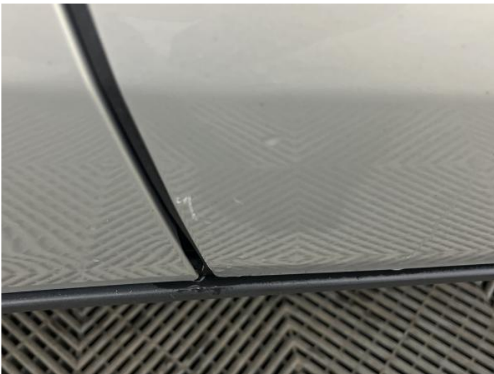
1: Door osf Scratched Over 25mm Thru Paint
