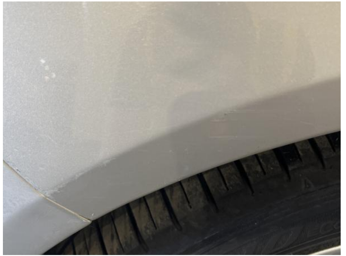
6: Wing nsf Scratched Over 25mm Thru Paint
