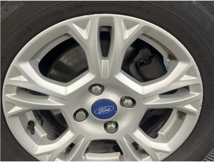
3: Wheel osf Corroded Light
