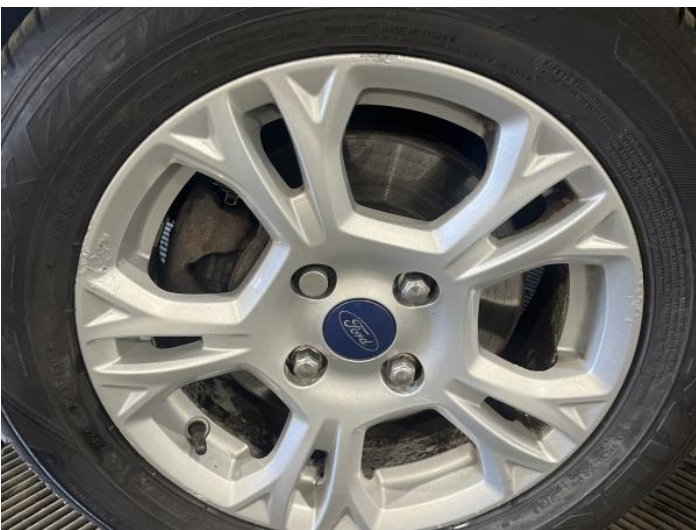
7: Wheel nsf Corroded Light
