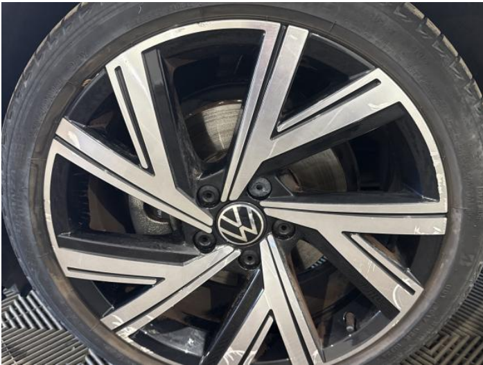
5: Wheel nsf Scratched Over 50mm
