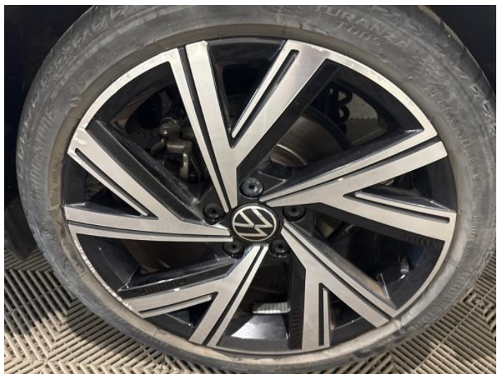
8: Wheel nsr Scratched Over 50mm
