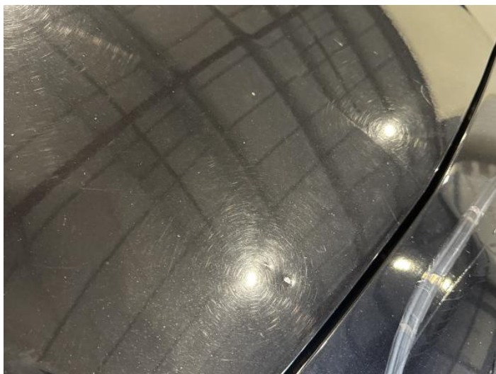
1: Bonnet Dented With Paint Damage
