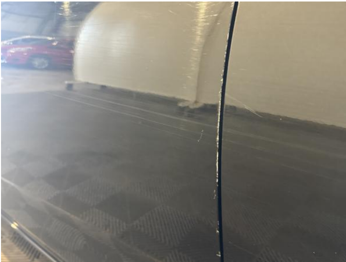
5: Door nsf Chipped Edge Chip
