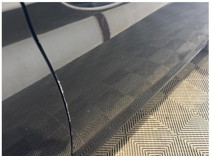
14: Door osf Dented With Paint Damage
