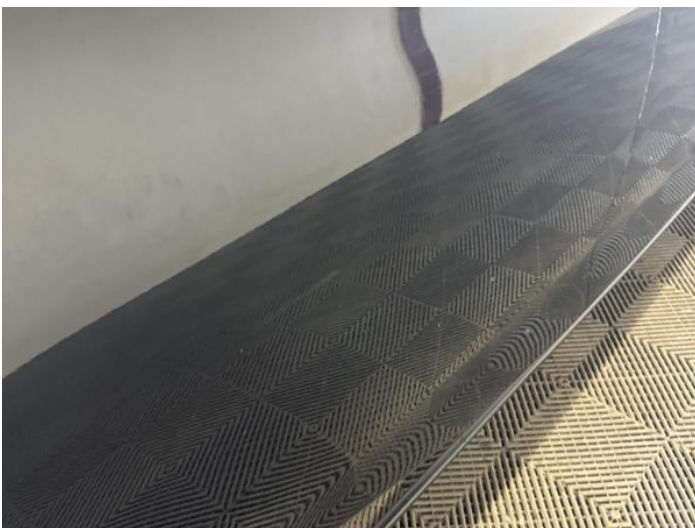
13: Door osr Scratched Over 25mm Thru Paint
