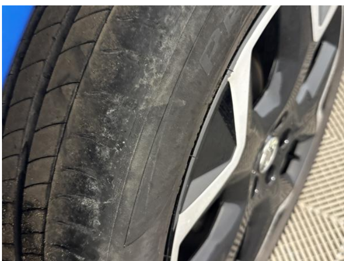
13: Tyre osr Damaged Replace
