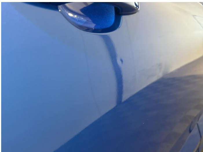
9: Door osr Dented Between 10mm + 30mm
