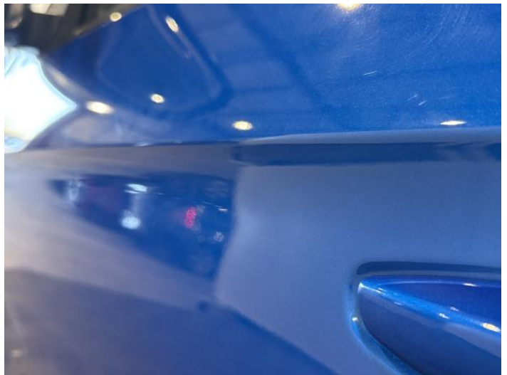
6: Door nsf Poor Previous Repair Poor Paint
