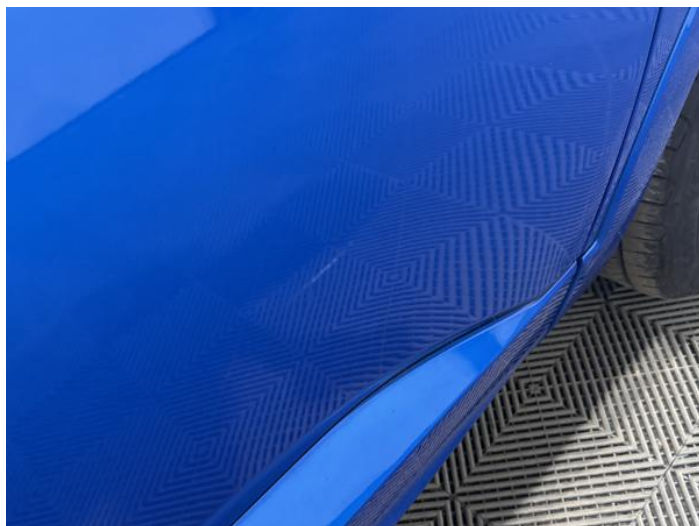
10: Door osf Scratched Over 25mm Thru Paint
