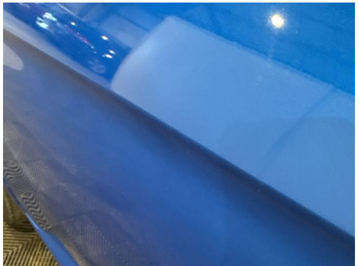
4: Door nsf Dented Between 10mm + 30mm
