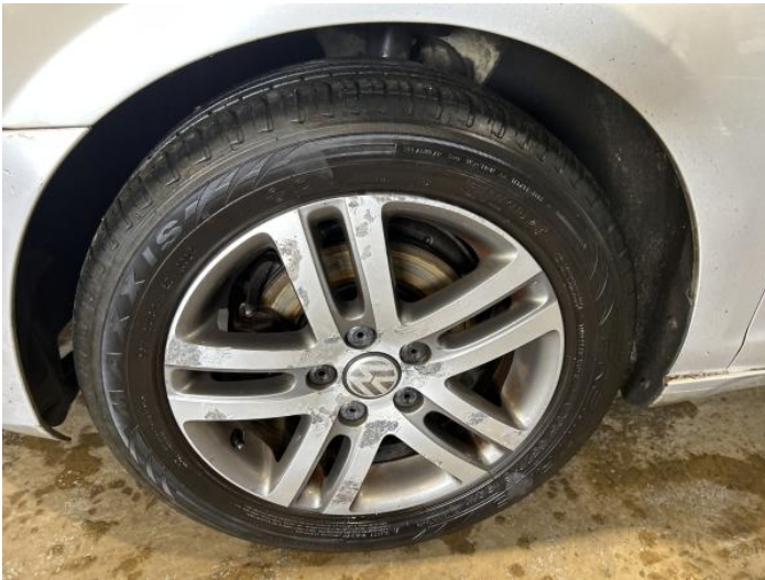
17: Wheel nsf Corroded Light
