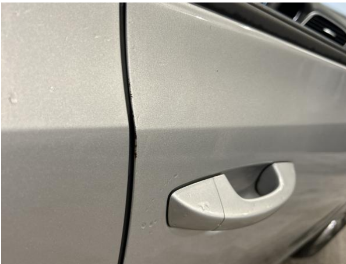
5: Door osf Chipped Edge Chip
