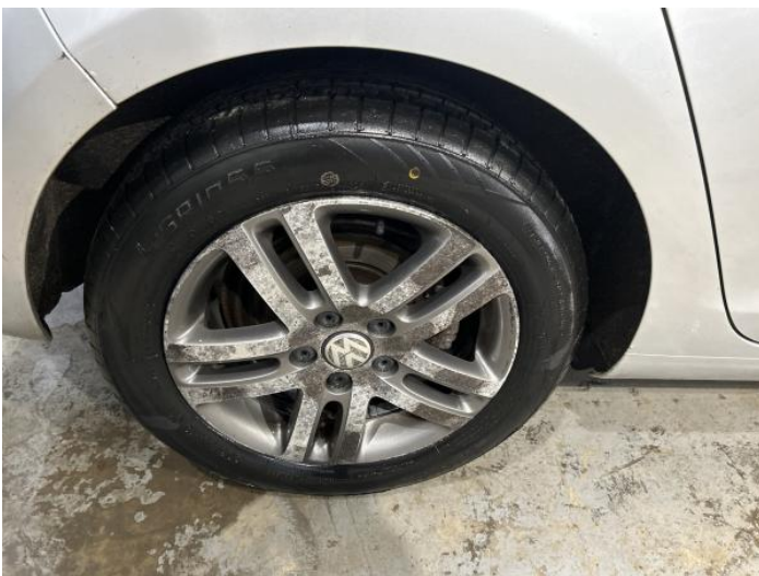
7: Wheel osr Corroded Light
