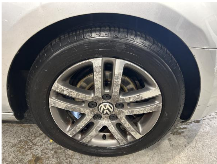
1: Wheel osf Corroded Light
