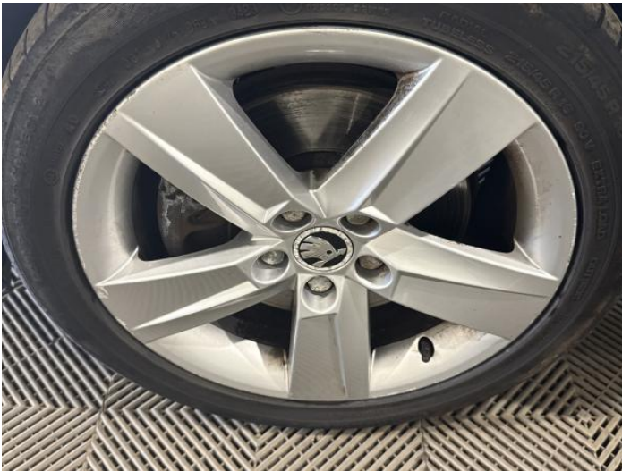
5: Wheel nsf Scratched Over 50mm
