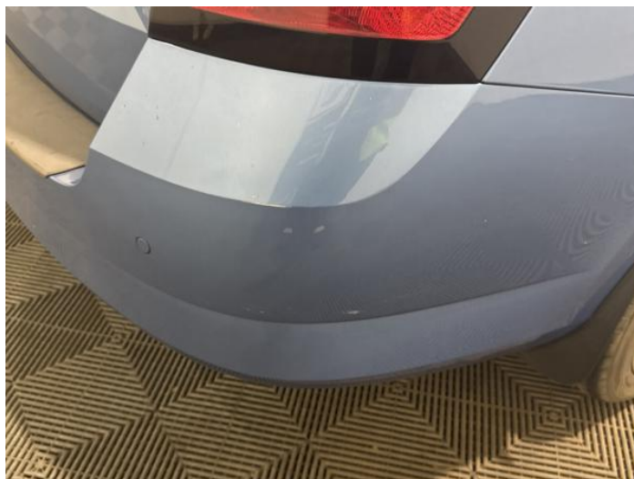
10: Bumper Rear Scratched 25 to 100mm Thru Paint
