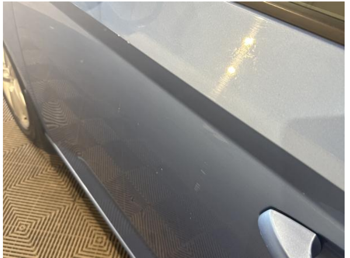
6: Door nsf Dented With Paint Damage
