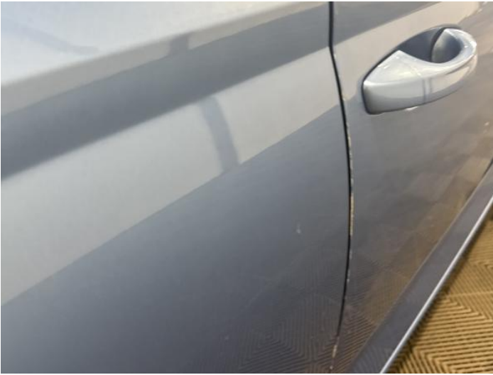
15: Door osr Dented Between 10mm + 30mm
