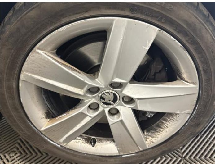
19: Wheel osf Scratched Over 50mm
