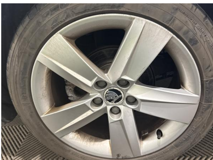
13: Wheel osr Scratched Up To 50mm
