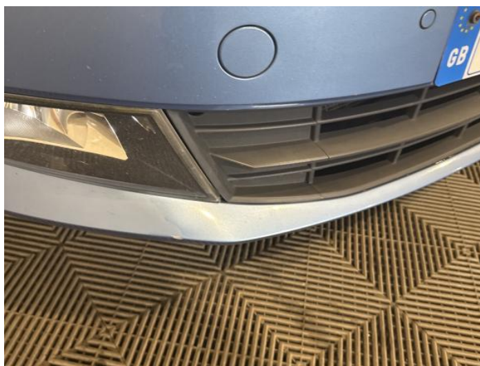
2: Bumper Front Dented With Paint Damage
