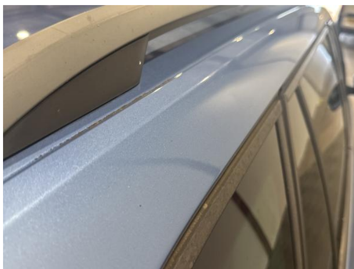
12: C Post os Dented Between 10mm + 30mm
