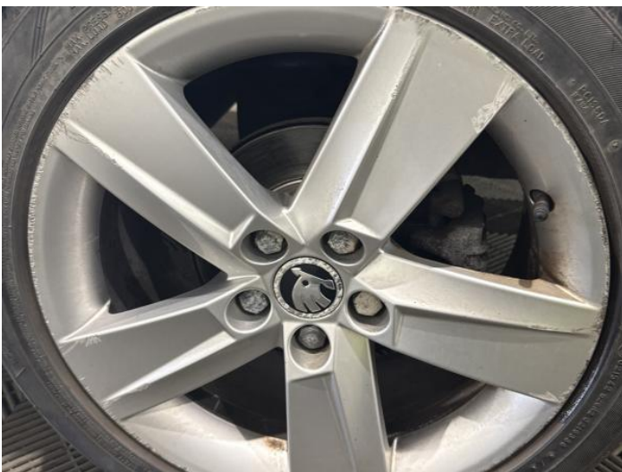
7: Wheel nsr Scratched Over 50mm
