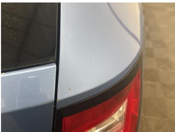
11: Qtr Panel osr Scratched Rusted
