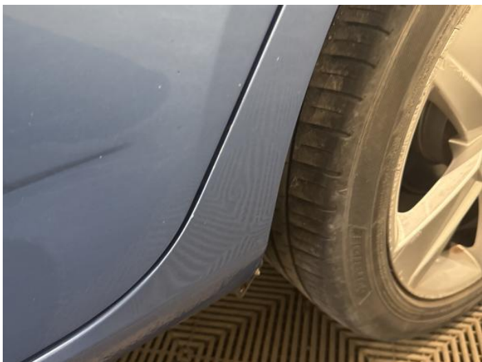
9: Qtr Panel nsr Dented With Paint Damage
