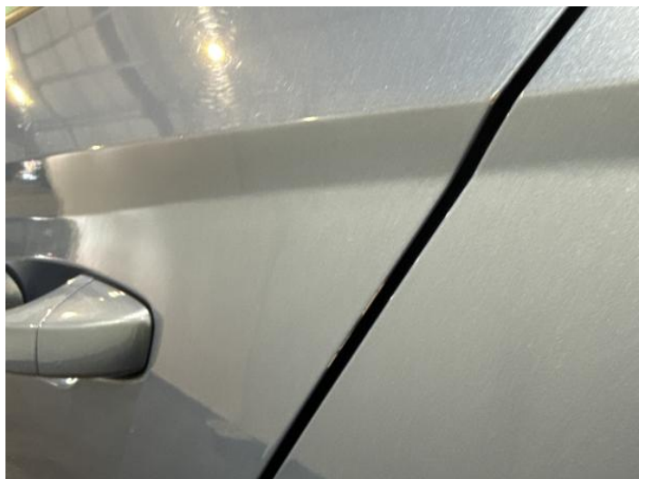
8: Door nsr Chipped Edge Chip
