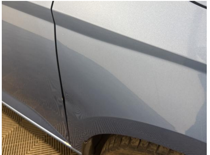
18: Wing nsf Dented Over 30mm
