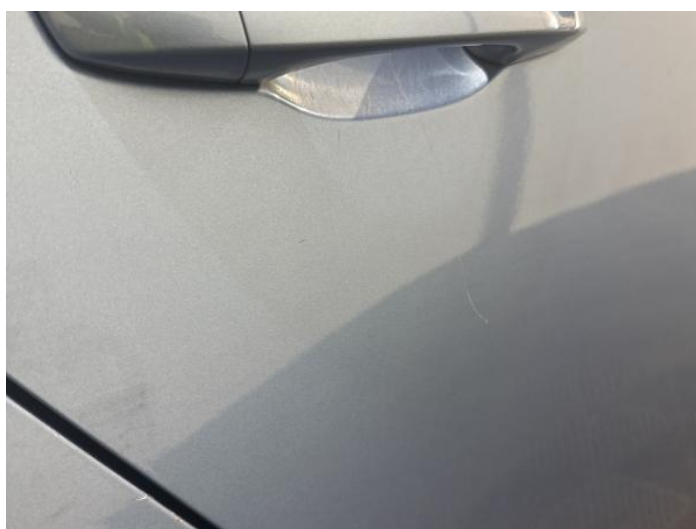
14: Door osr Scratched UpTo 25mm Thru Paint
