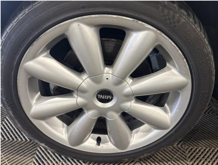
3: Wheel nsf Scratched Over 50mm
