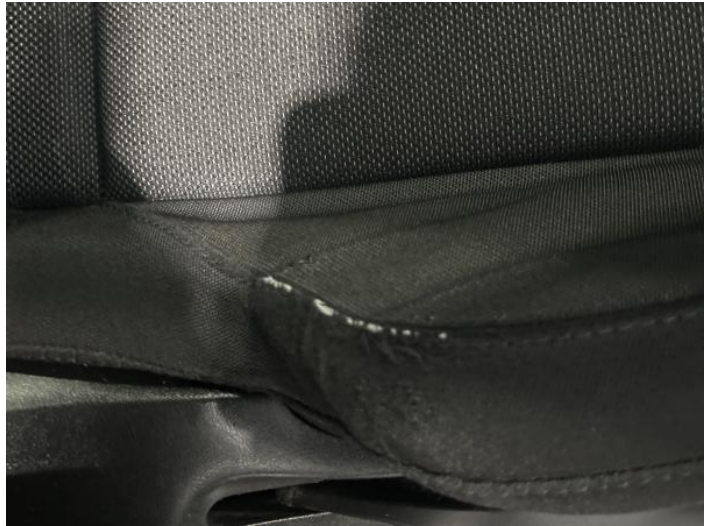
22: Seat Base Cover osf Scuffed UpTo 25mm
