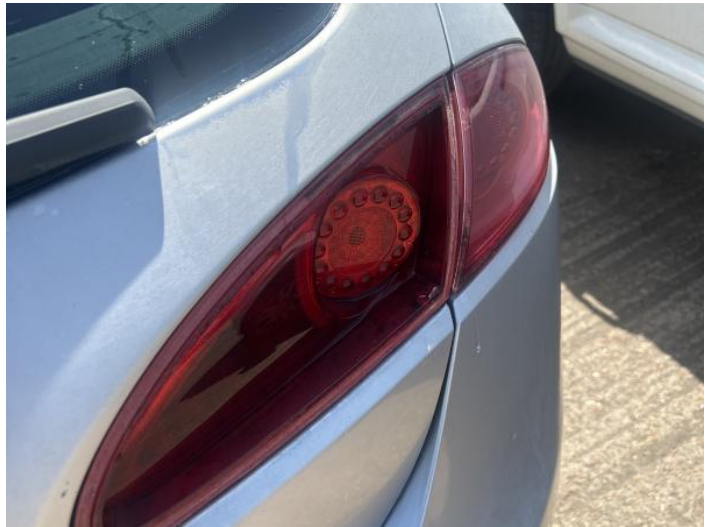
18: Lamp osr Broken Replace
