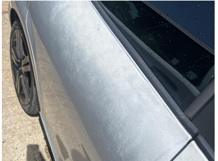
4: Door osr Poor Previous Repair Poor Paint
