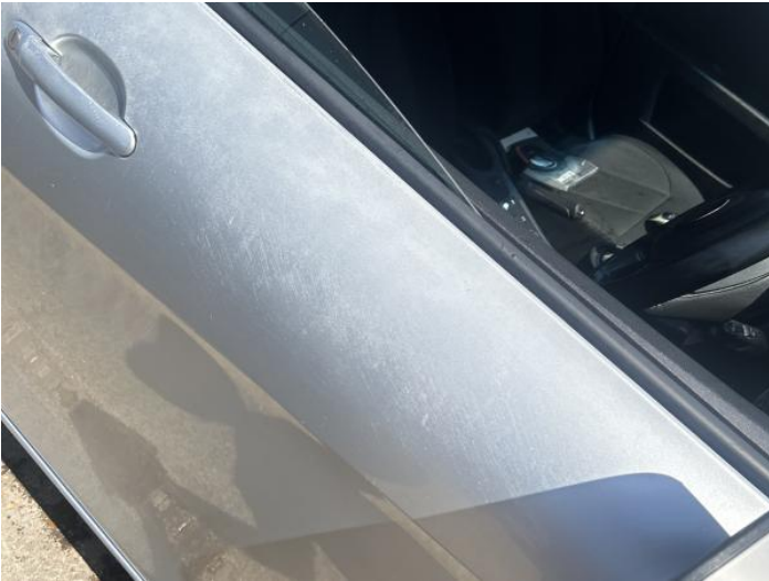
3: Door osf Poor Previous Repair Poor Paint
