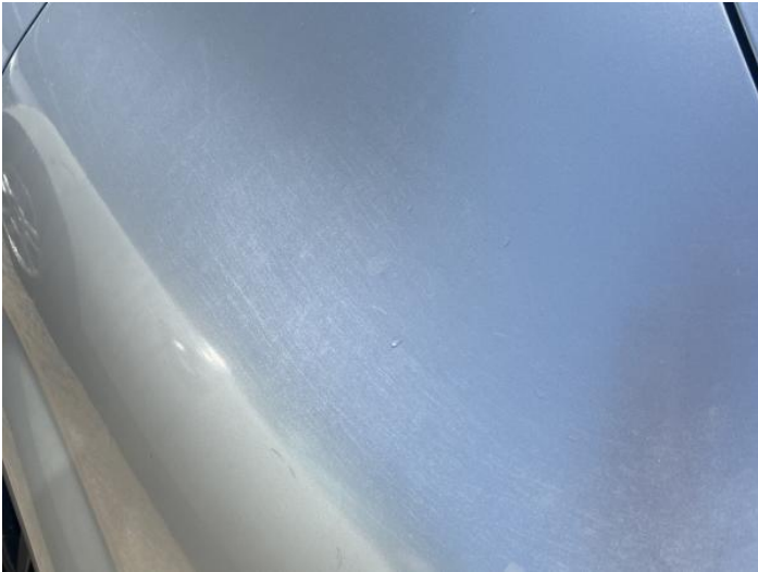
9: Qtr Panel nsr Poor Previous Repair Poor Paint
