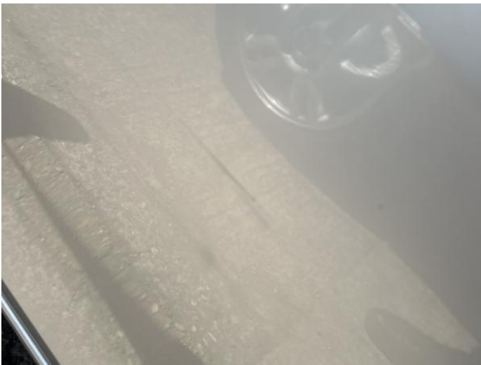
11: Door nsr Scratched Over 25mm Thru Paint
