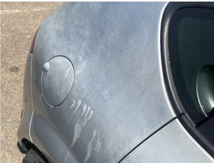
5: Qtr Panel osr Poor Previous Repair Poor Paint
