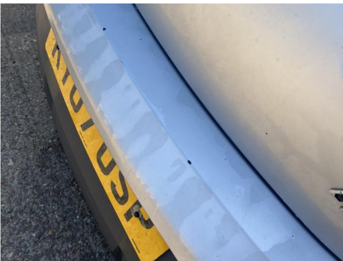
7: Bumper Rear Poor Previous Repair Poor Paint
