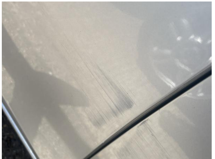
12: Door nsf Scratched Over 25mm Thru Paint
