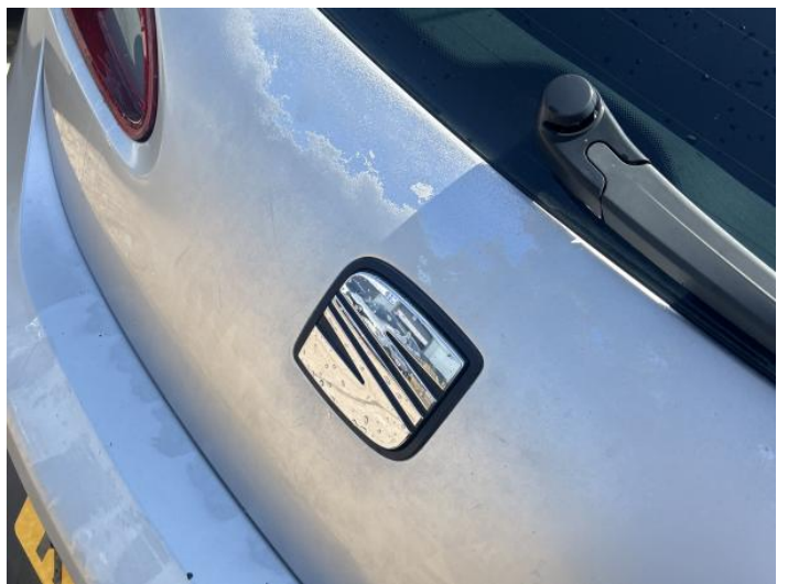
8: Tailgate Poor Previous Repair Poor Paint
