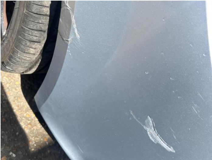
15: Bumper Front Cracked Over 25mm
