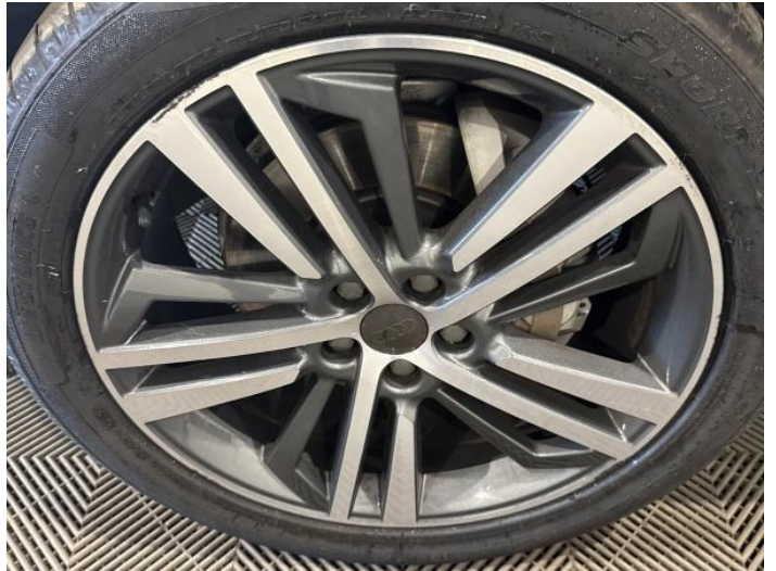
4: Wheel nsf Scratched Over 50mm
