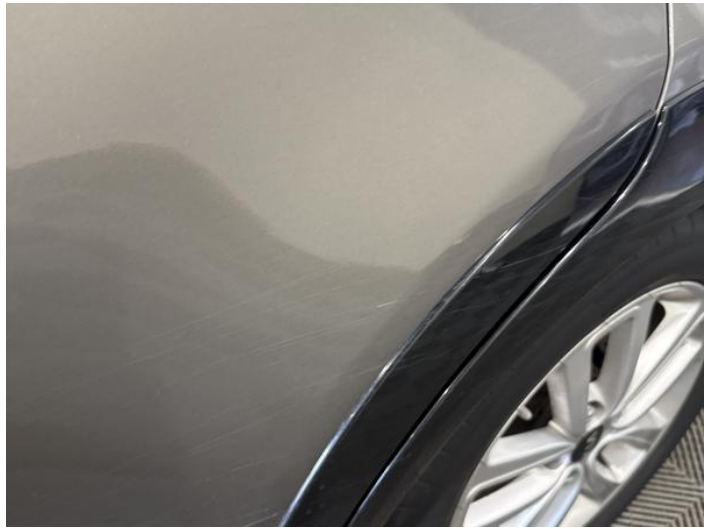
6: Door nsr Scratched Over 25mm Thru Paint
