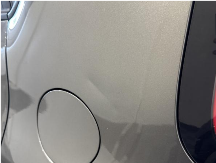
15: Qtr Panel nsr Dented Over 30mm
