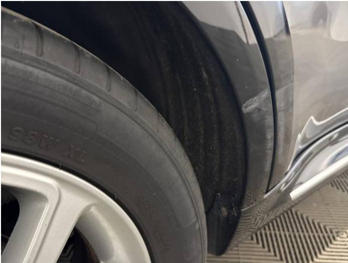
9: Qtr Panel Arch Extension os Scratched (Painted) Over 25mm Thru Paint
