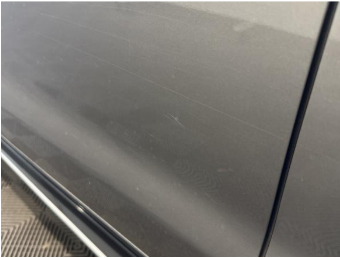
5: Door nsf Scratched UpTo 25mm Thru Paint
