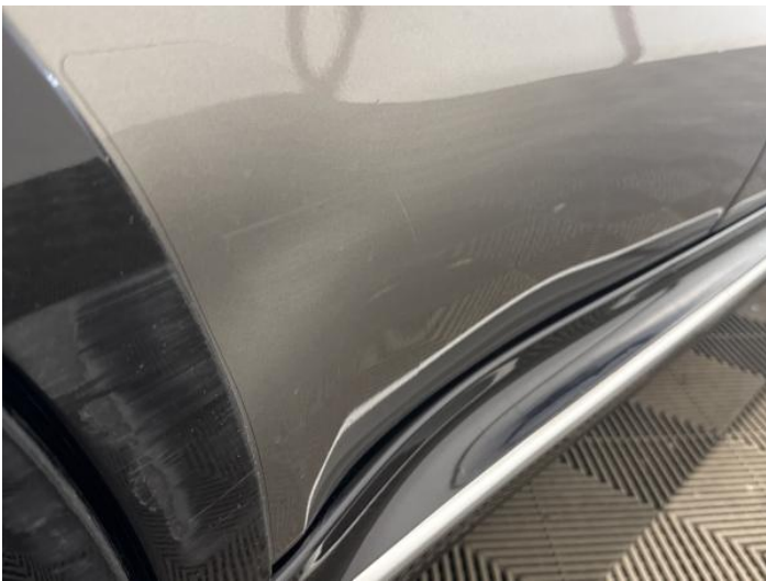
11: Door osr Scratched Over 25mm Thru Paint
