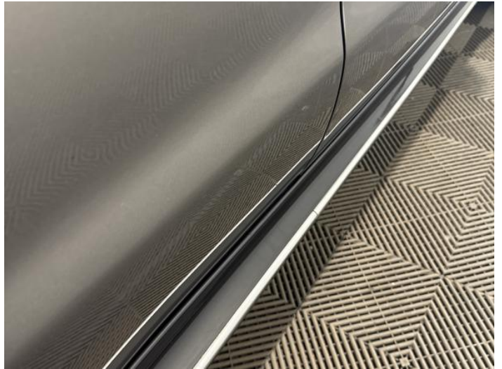
10: Door osr Dented Between 10mm + 30mm
