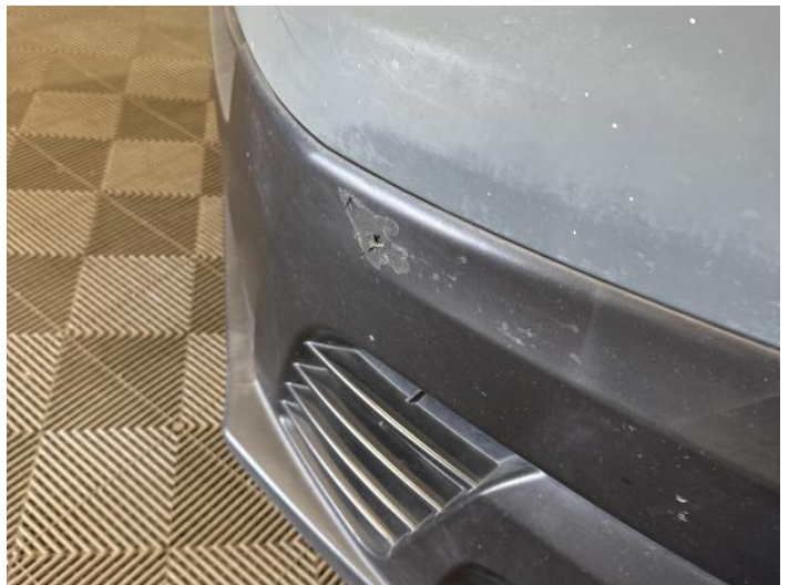
2: Bumper Front Moulding Scuffed (Unpainted) UpTo 100mm
