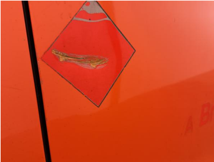
9: Door osf Dented With Paint Damage
