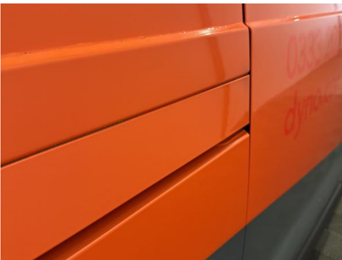
7: Qtr Panel osr Dented Between 10mm + 30mm
