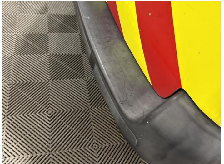
6: Bumper Rear Moulding Scuffed (Unpainted) Up To 100mm
