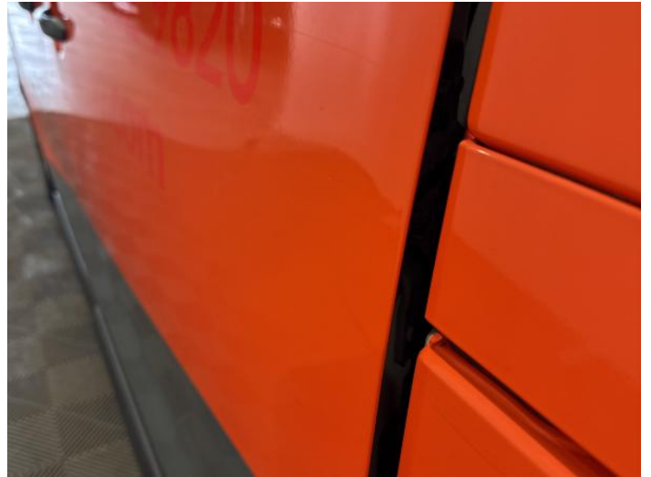
4: Door nsf Dented Over 30mm
