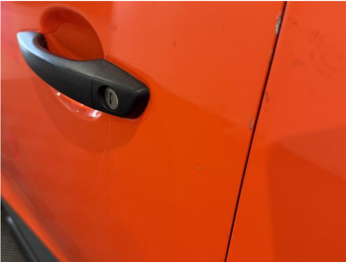
3: Door nsf Chipped 1 To 5
