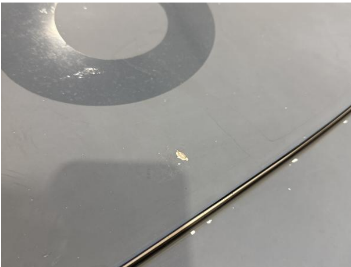
1: Bonnet Scratched UpTo 25mm Thru Paint
