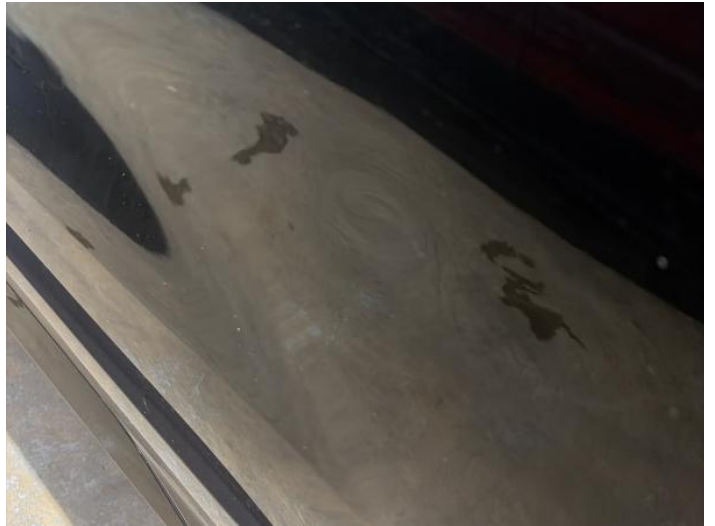
4: Door nsr Dented Over 30mm
