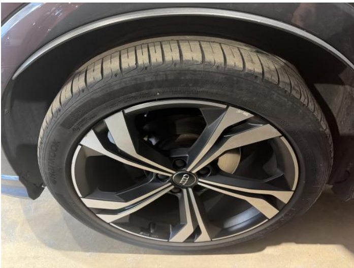
5: Wheel nsf Corroded Light
