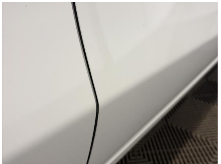
14: Door osf Chipped Edge Chip
