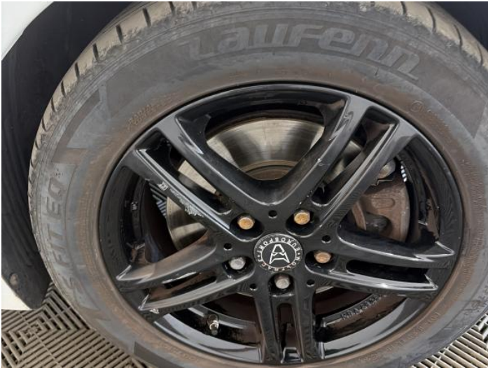
15: Wheel osf Scratched Over 50mm
