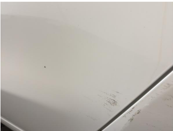
7: Door nsr Scratched Over 25mm Thru Paint
