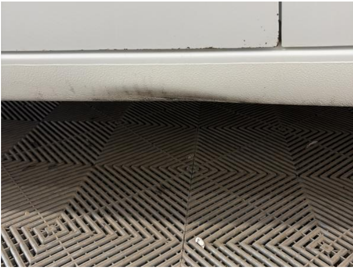
5: Sill ns Dented Over 30mm
