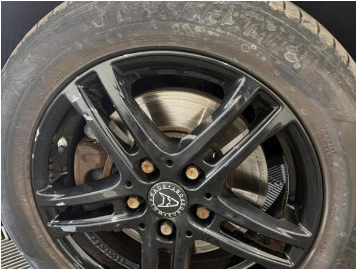
3: Wheel nsf Scratched Over 50mm
