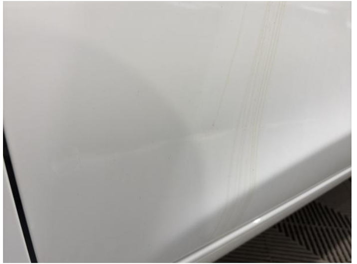
4: Door nsf Dented Over 30mm
