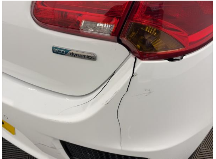
10: Bumper Rear Cracked Over 25mm
