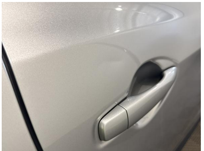
14: Door osr Dented Over 30mm
