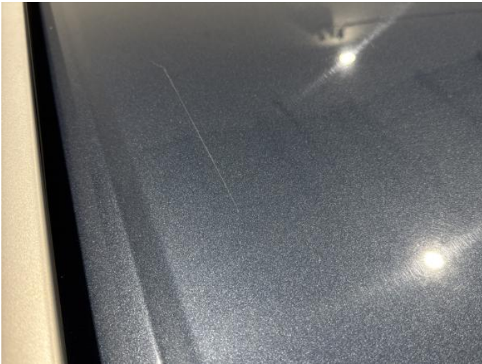
17: Roof Scratched Over 25mm Thru Paint
