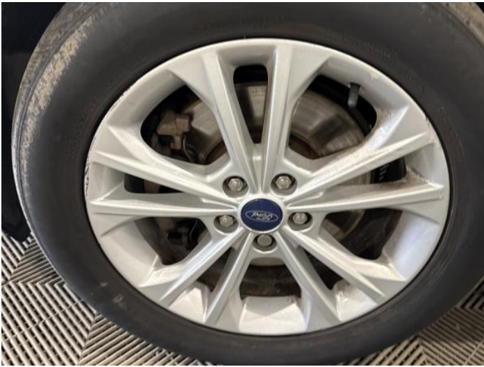
5: Wheel nsf Scratched Over 50mm
