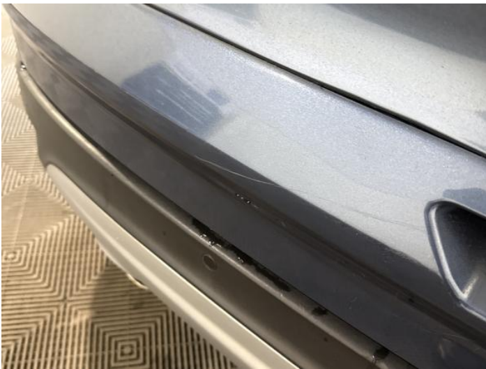
11: Tailgate Scratched Over 25mm Thru Paint
