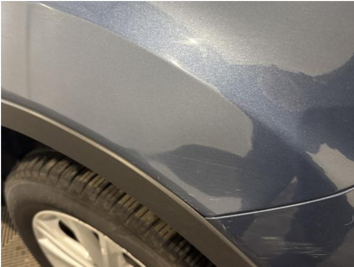
9: Qtr Panel nsr Dented Over 30mm
