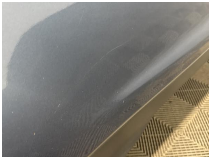
14: Door osr Scratched Over 25mm Thru Paint
