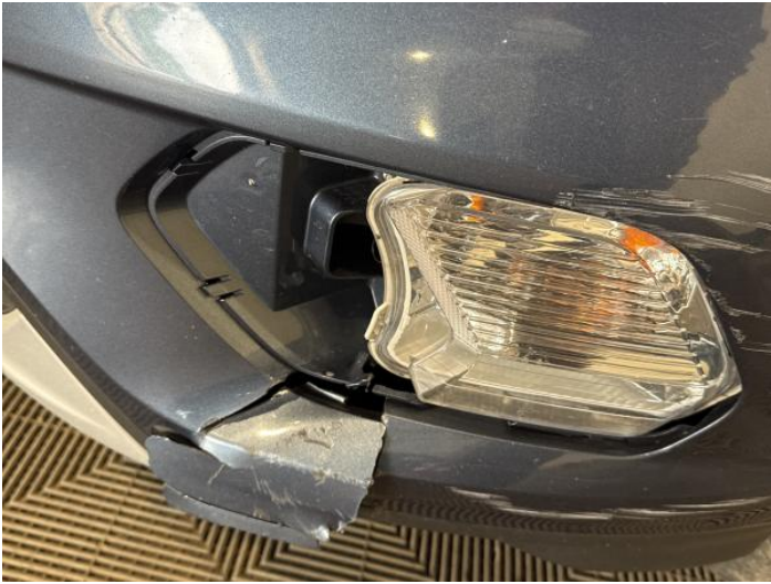
3: Fog Lamp Surround ns Broken Replace
