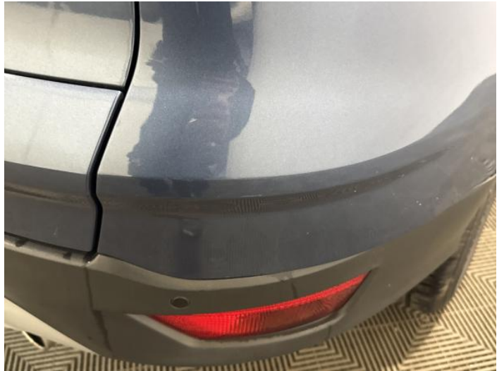
10: Bumper Rear Scratched 25 to 100mm Thru Paint
