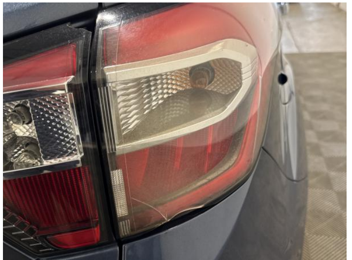
12: Lamp nsr Broken Replace
