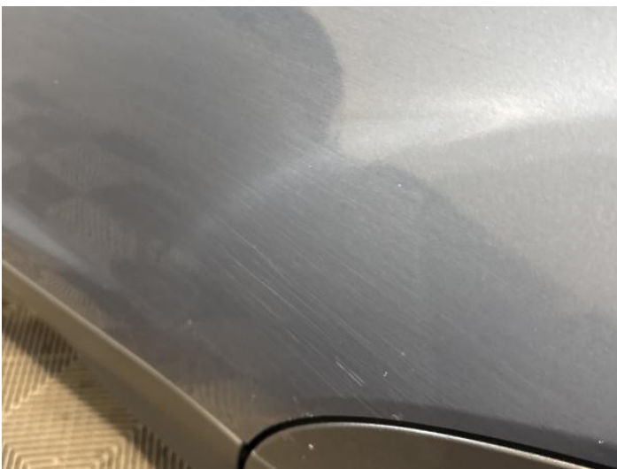
7: Door nsr Scratched Over 25mm Thru Paint
