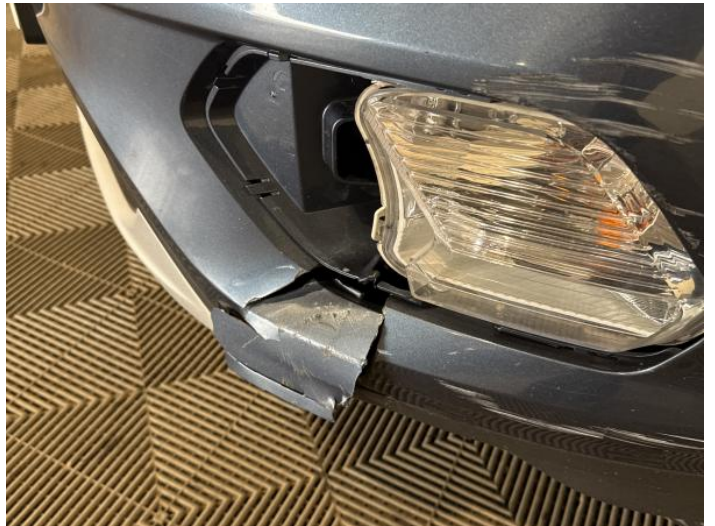
2: Bumper Front Cracked Over 25mm
