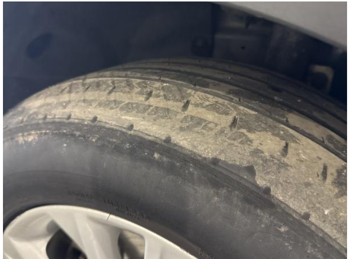
18: Tyre nsf Damaged Replace
