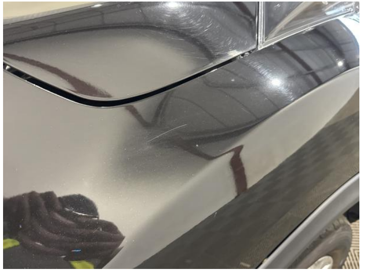
12: Wing osf Scratched Over 25mm Thru Paint
