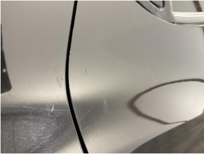
9: Door osr Chipped Edge Chip
