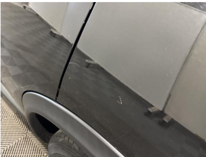
7: Qtr Panel nsr Scratched Up To 25mm Thru Paint
