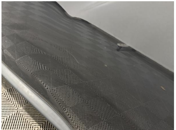
6: Door nsr Scratched Over 25mm Thru Paint
