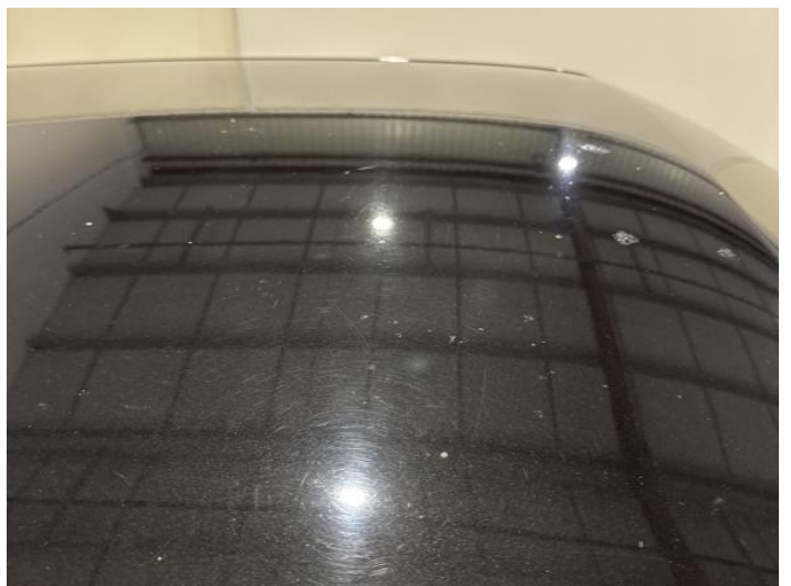
14: Roof Scratched Over 25mm Thru Paint
