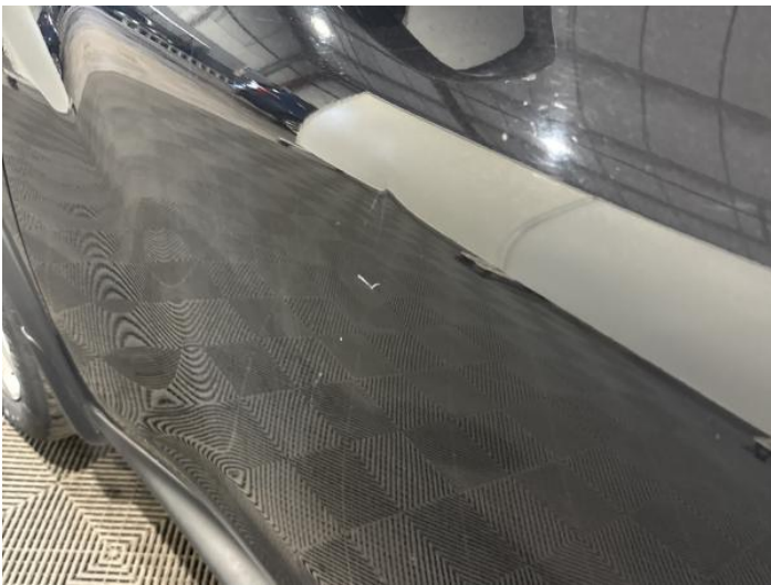
5: Door nsf Dented With Paint Damage
