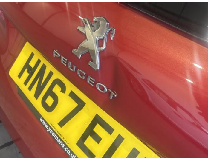
7: Tailgate Dented Over 30mm
