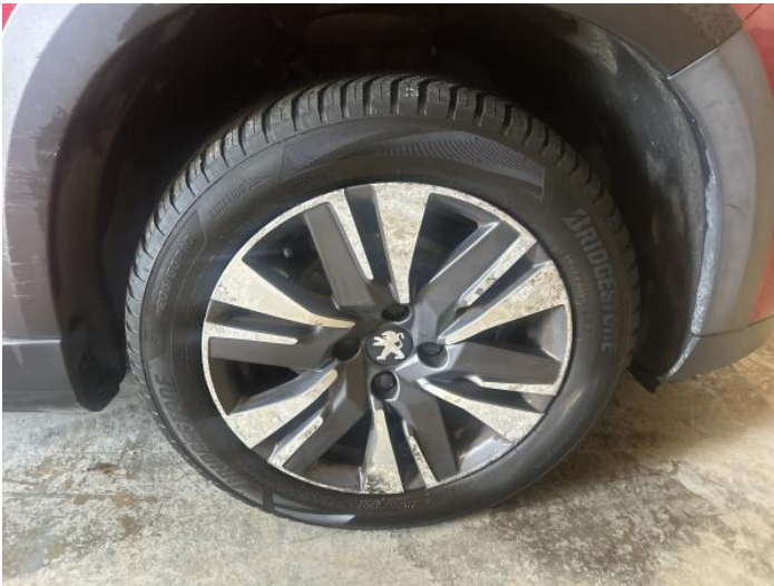
1: Wheel osf Corroded Light
