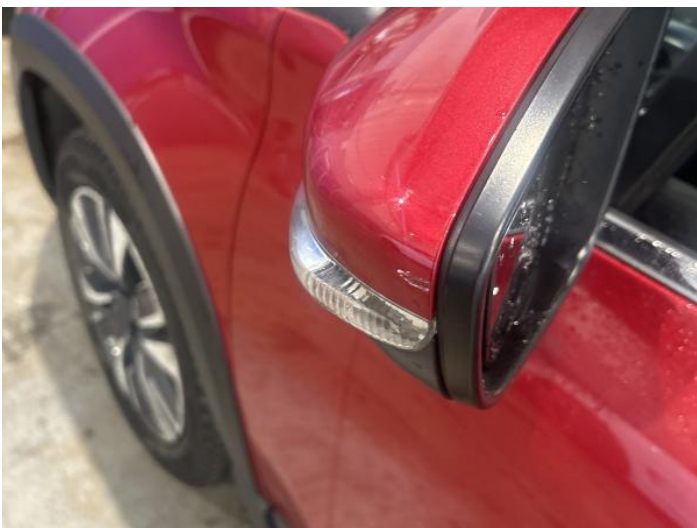
13: Door Mirror Assy nsf Scratched (Painted) UpTo 25mm Thru Paint
