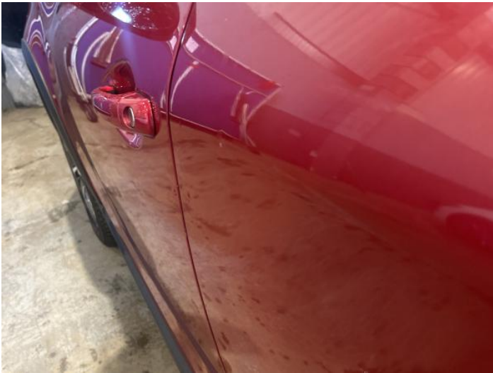
11: Door nsr Dented 2 Or Less UpTo 10mm
