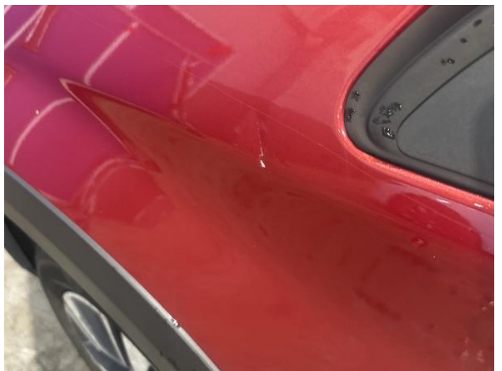
14: Wing nsf Dented With Paint Damage
