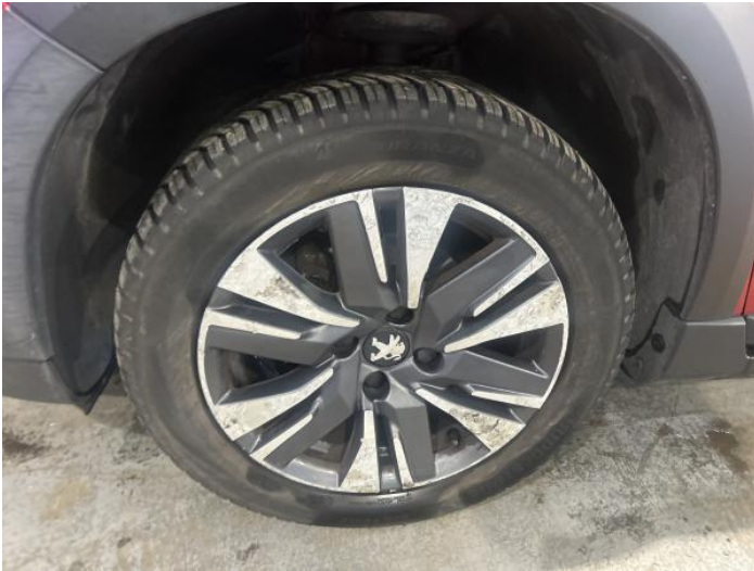
15: Wheel nsf Corroded Light
