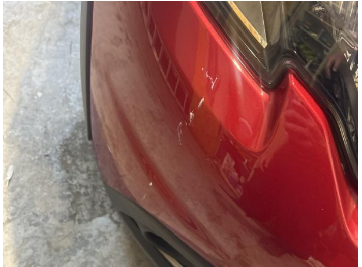
16: Bumper Front Scratched 25 to 100mm Thru Paint
