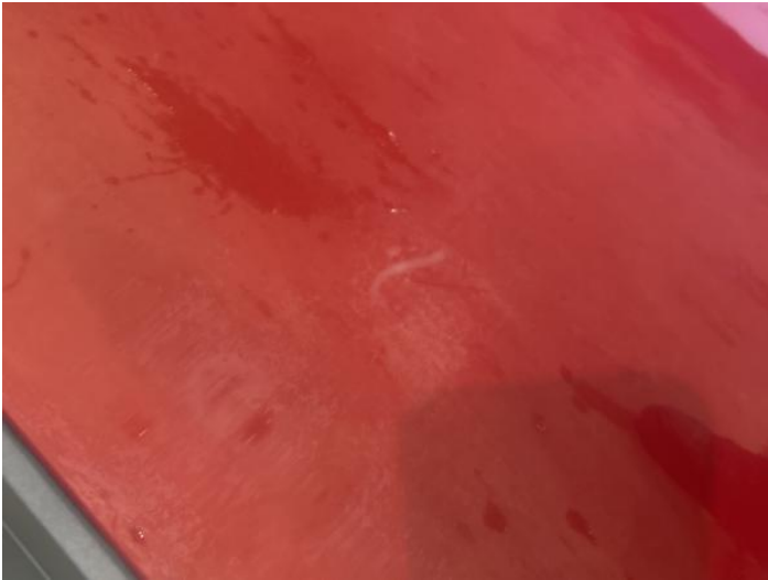
9: Door nsr Scratched UpTo 25mm Thru Paint
