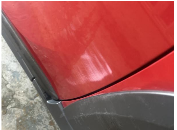
2: Door osf Scratched Over 25mm Thru Paint
