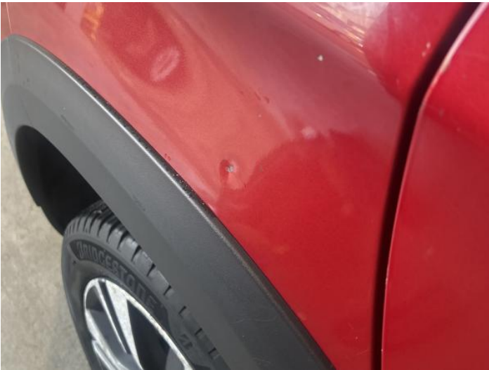
5: Qtr Panel osr Dented With Paint Damage
