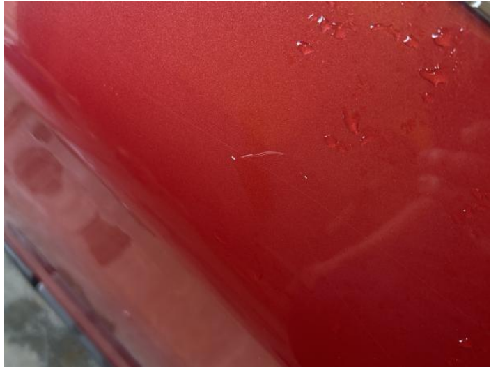
4: Door osr Scratched Up To 25mm Thru Paint
