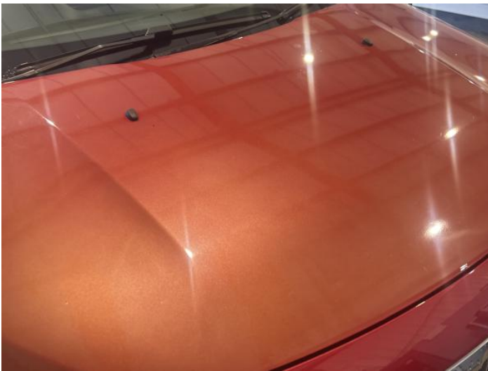
17: Bonnet Poor Previous Repair Poor Colour
