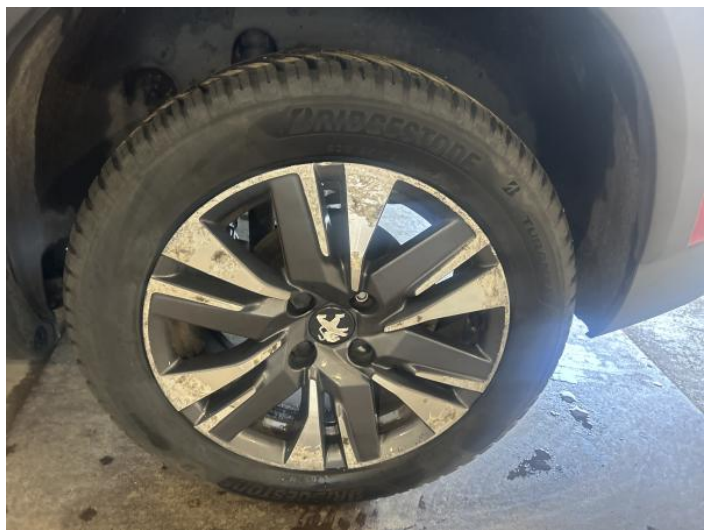
8: Wheel nsr Corroded Light
