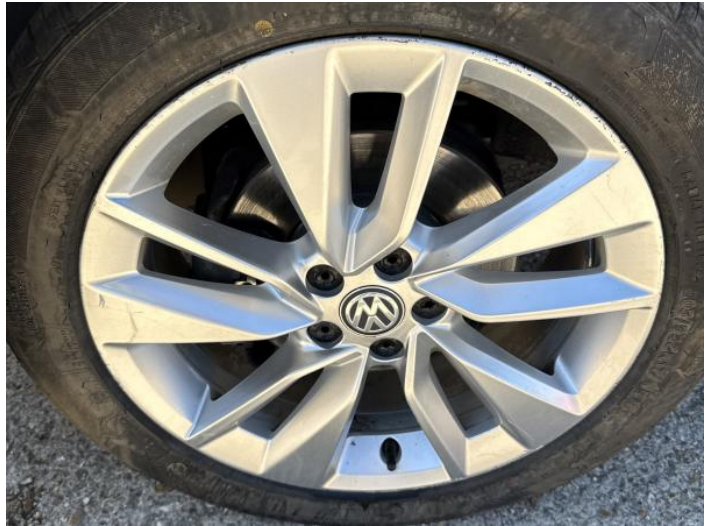
4: Wheel nsf Scratched Over 50mm
