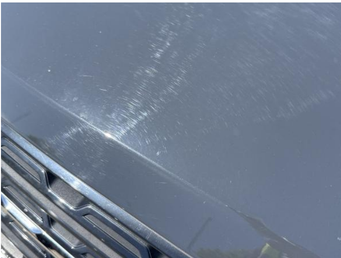
1: Bonnet Chipped Multiple Chips
