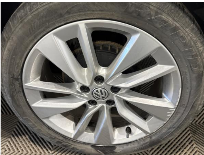
7: Wheel nsr Scratched Over 50mm
