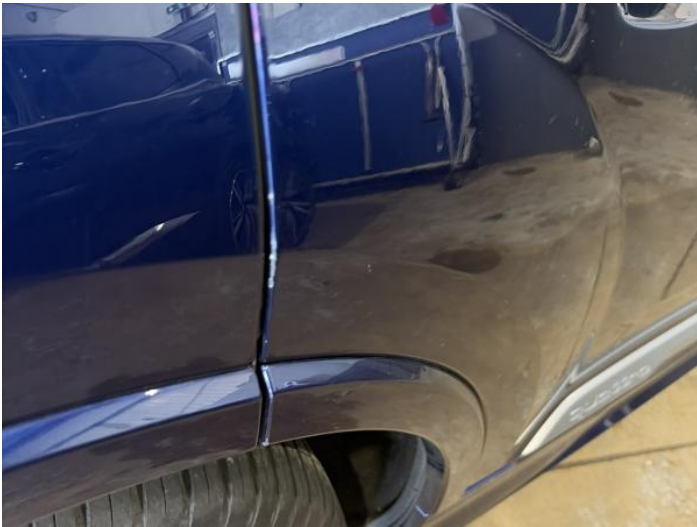
5: Door osr Chipped Edge Chip
