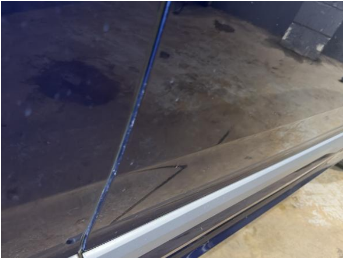
3: Door osf Chipped Edge Chip
