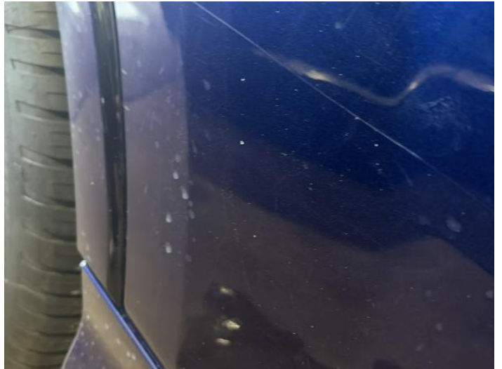
4: Door osr Chipped 1 To 5
