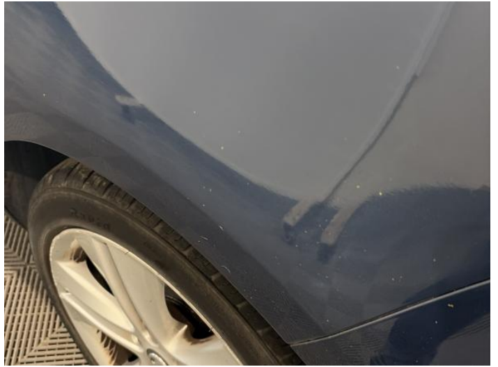
10: Qtr Panel nsr Scratched UpTo 25mm Thru Paint
