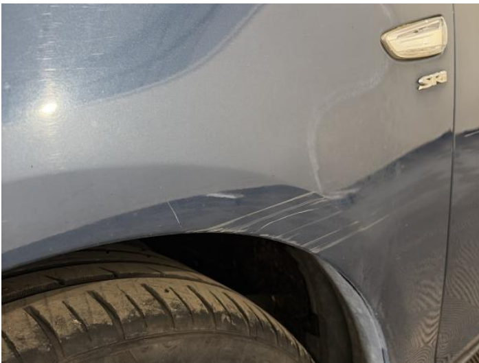
5: Wing nsf Scratched Over 25mm Thru Paint
