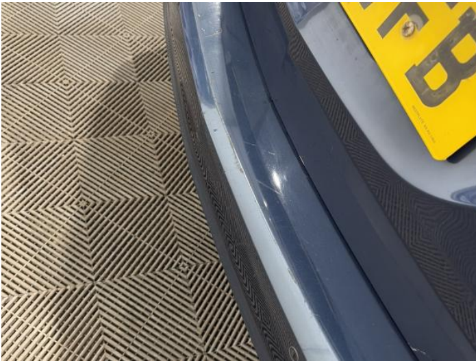
11: Bumper Rear Scratched 25 to 100mm Thru Paint
