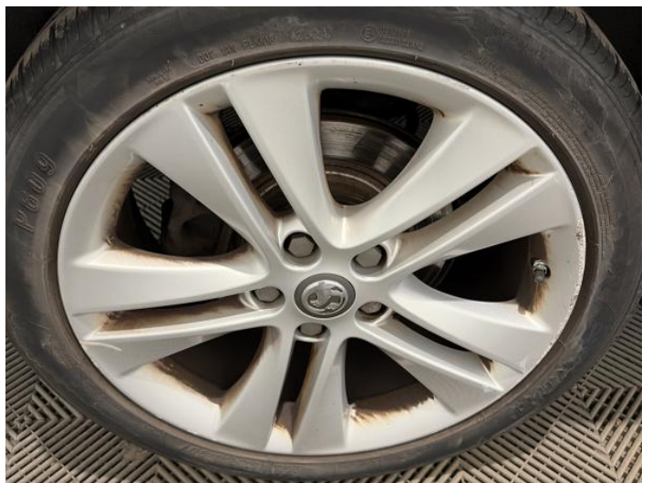
14: Wheel osr Scratched Over 50mm
