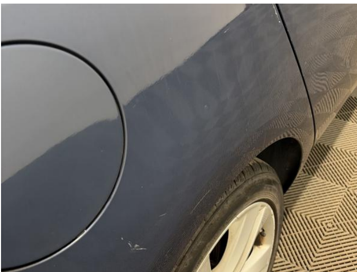
13: Qtr Panel osr Dented With Paint Damage
