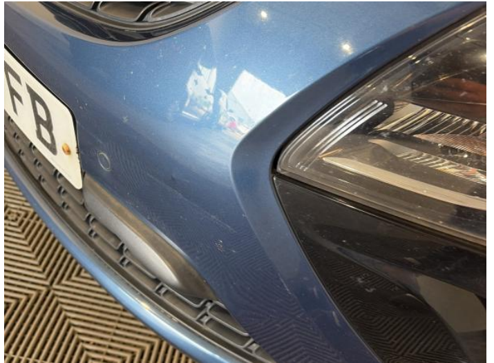
4: Bumper Front Dented With Paint Damage
