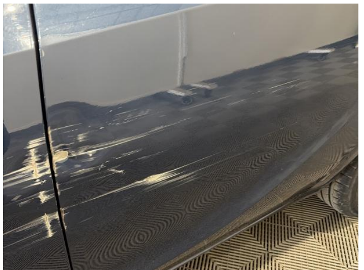
8: Door nsr Dented With Paint Damage
