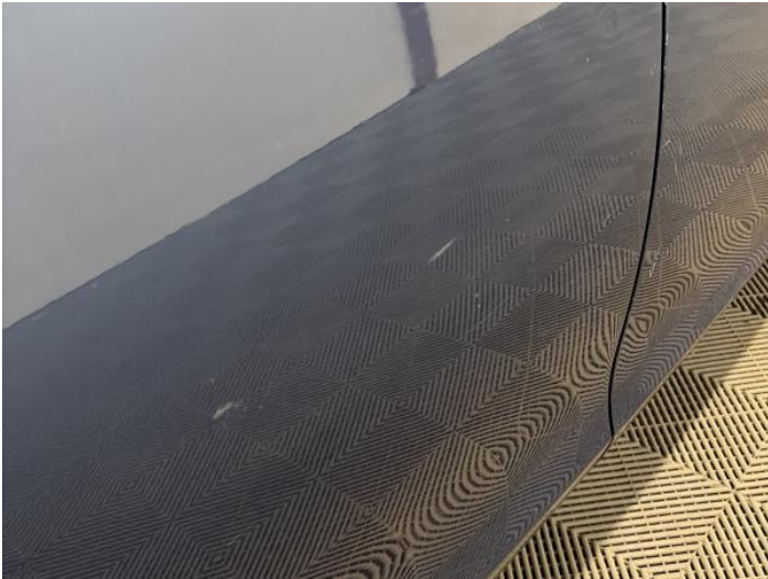
15: Door osr Scratched Over 25mm Thru Paint
