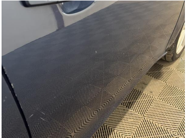
16: Door osf Scratched Over 25mm Thru Paint
