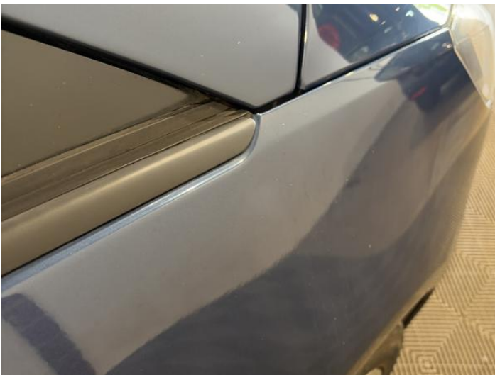
17: Wing osf Dented Over 30mm
