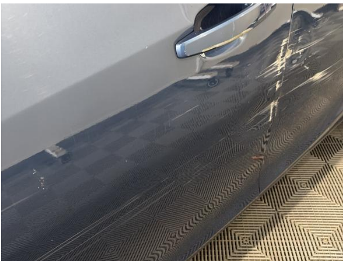
7: Door nsf Dented With Paint Damage
