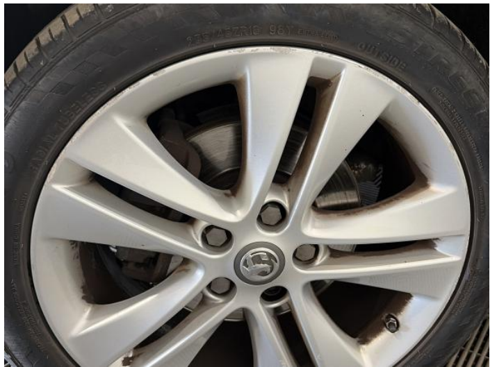
6: Wheel nsf Scratched Over 50mm
