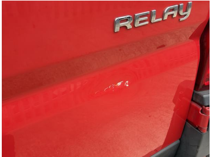
10: Tailgate Dented With Paint Damage
