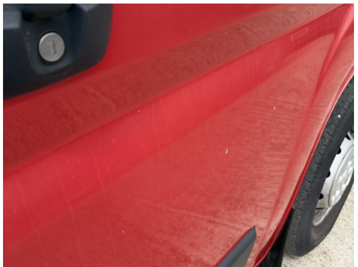
14: Door osf Dented 2 Or Less Up To 10mm
