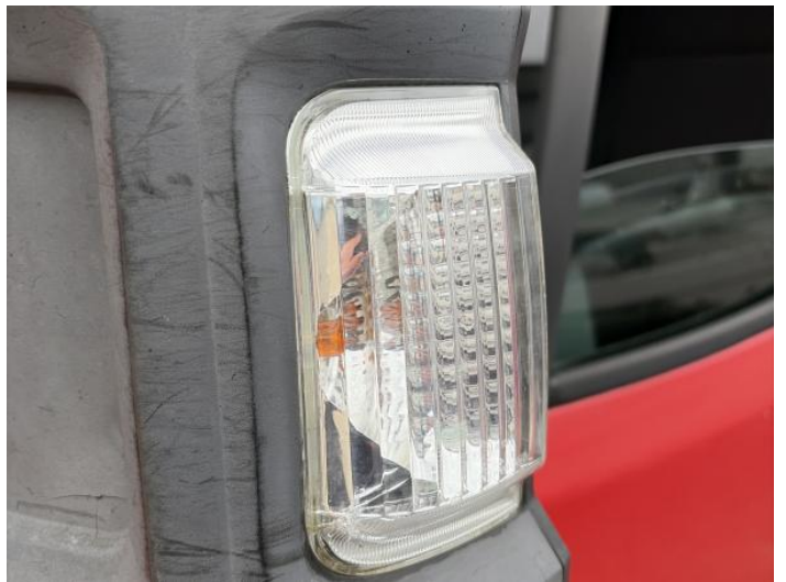
6: Flasher Side Repeater ns Broken Replace
