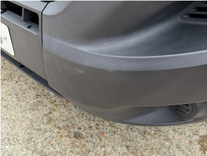
3: Bumper Front Moulding Scuffed (Unpainted) Over 100mm
