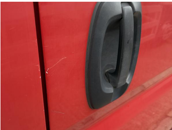
7: Door nsr Scratched Over 25mm Thru Paint
