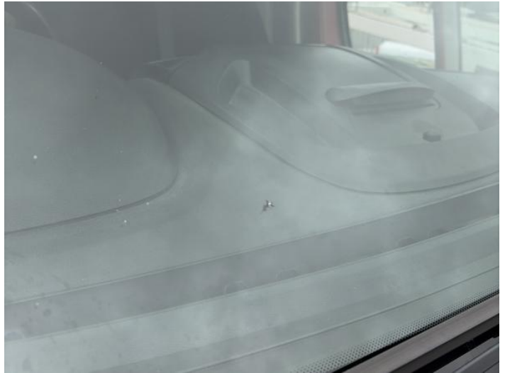
16: Screen Front Chipped Over 10mm
