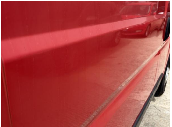
12: Panel Front Dented Over 30mm
