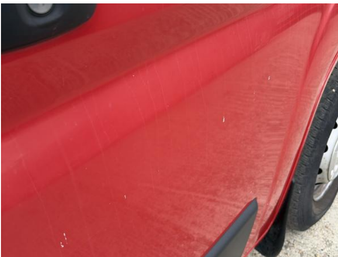
13: Door osf Scratched Over 25mm Thru Paint
