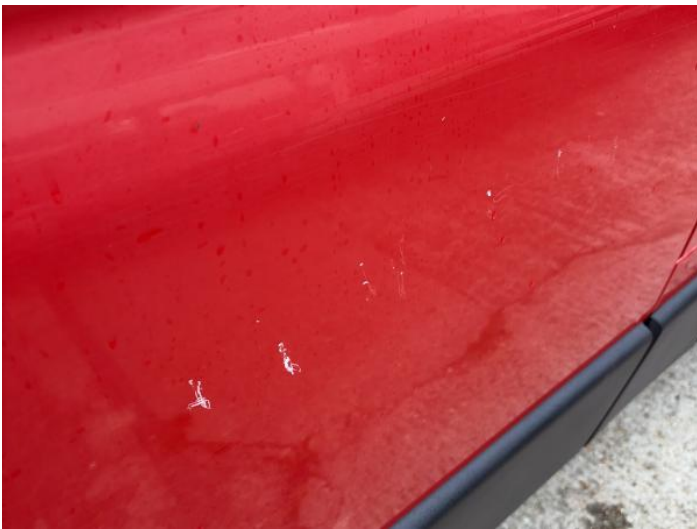
5: Door nsf Scratched Over 25mm Thru Paint
