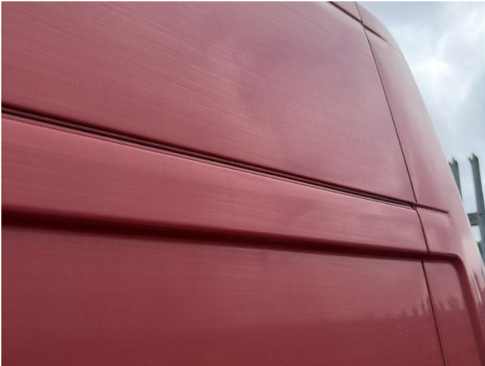
9: Qtr Panel nsr Dented Over 30mm
