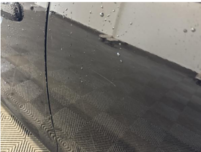
7: Door nsr Scratched Over 25mm Thru Paint
