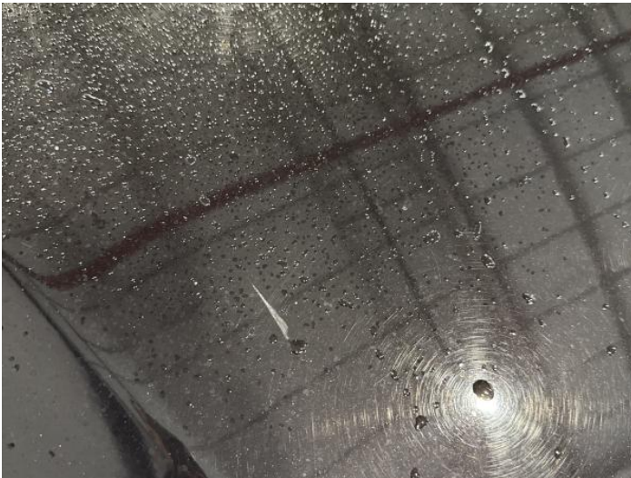
1: Bonnet Scratched Over 25mm Thru Paint
