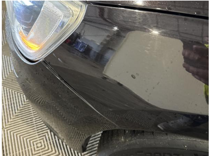
4: Wing nsf Scratched Over 25mm Thru Paint
