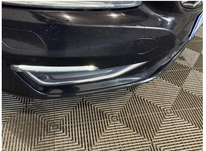
2: Bumper Front Scratched Over 100mm Thru Paint
