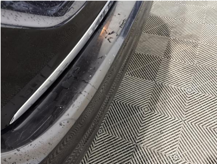
9: Bumper Rear Scratched 25 to 100mm Thru Paint
